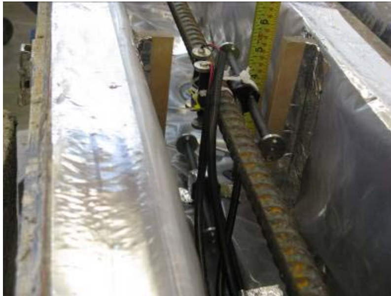
(b) Installed VWSGs
