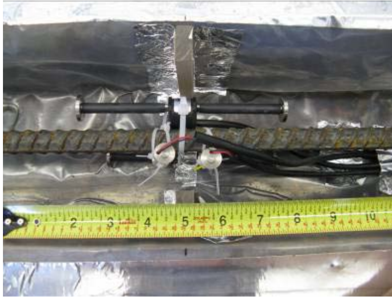
(a) Plan view of installed VWSGs
