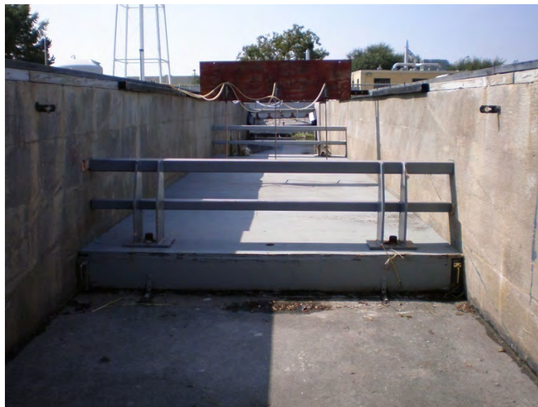
Figure 3.18: Model Wyoming Bridge Rails in Series Looking Downstream
