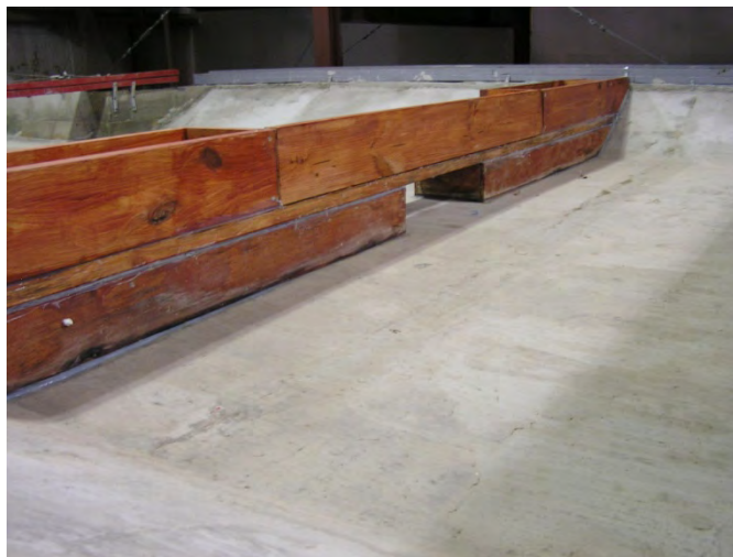
Figure 3.26: Temporary obstruction used to establish an underflow rating curve
