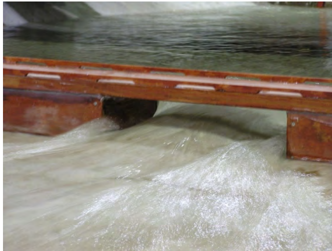
Figure 3.25: Model with two 30% open space railings
