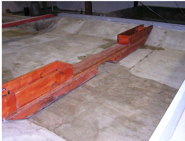
Figure 3.22: Model bridge deck looking downstream
