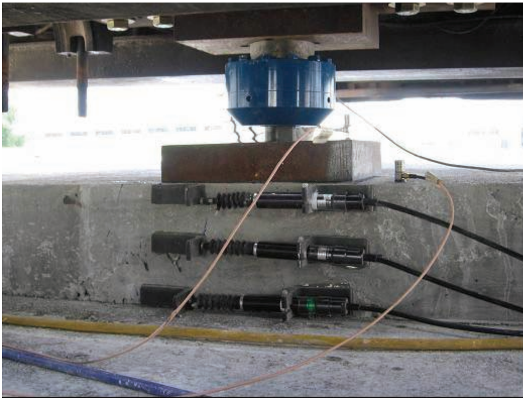
Figure 4.20: Arrangement of loading frame and LVDTs
