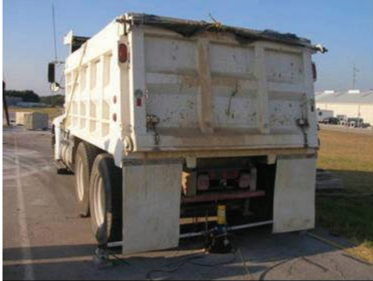
(a) Plate load test using fully loaded dump truck
