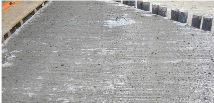
Figure 4.8: Broom Finish Produced in Laboratory
