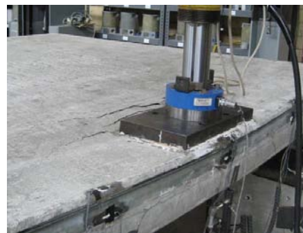
Figure 5.3: Response of Specimen 1 during Static Test to Failure
