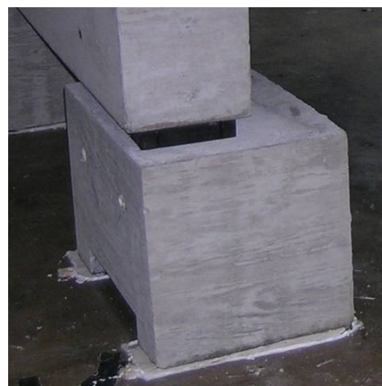
Figure 4.3: Cross Section and Support of Precast Beams
