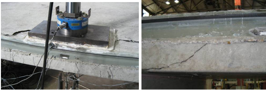
Figure 5.7: Photographs of Specimen 2 after Punching Shear Failure
