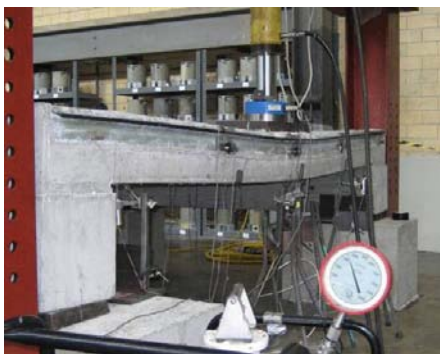
Figure 5.3: Response of Specimen 1 during Static Test to Failure
