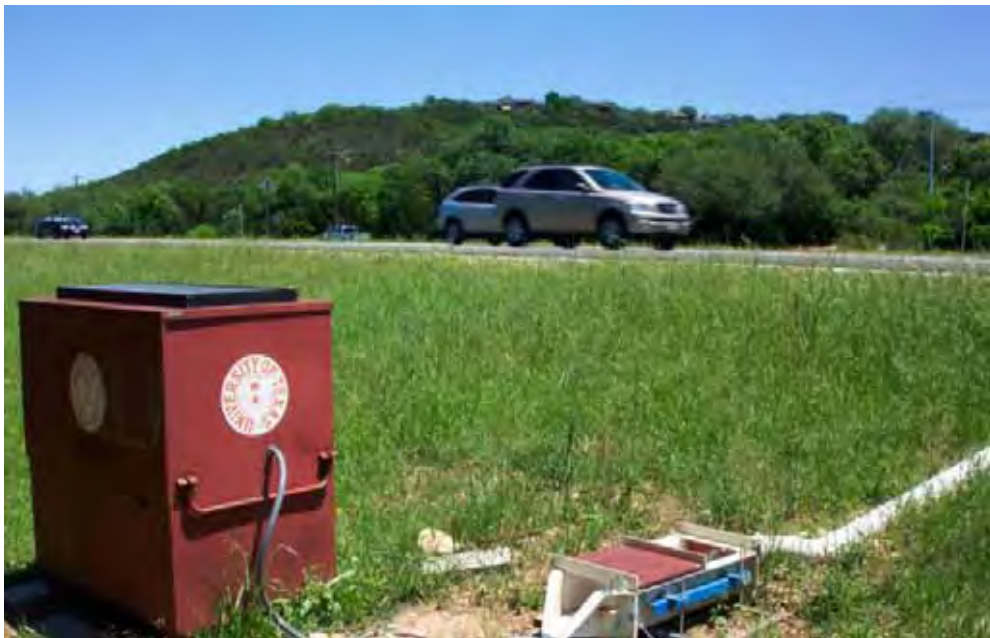
Figure 5-33: Photograph of H-flume and drainage pipe at Loop 360 monitoring site
