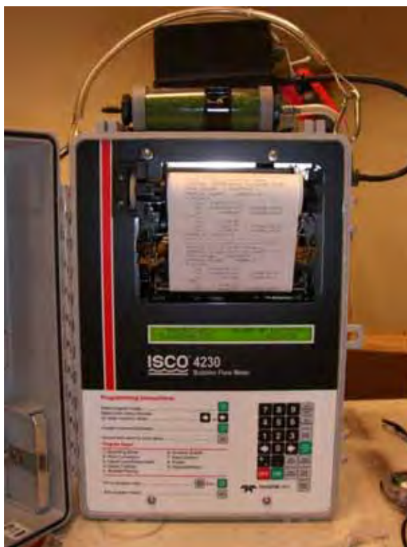
Figure 3-13: ISCO bubbler used to measure standpipe head
