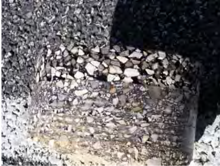
Figure 3-5: Extracted PFC core with porous layer and impermeable base
