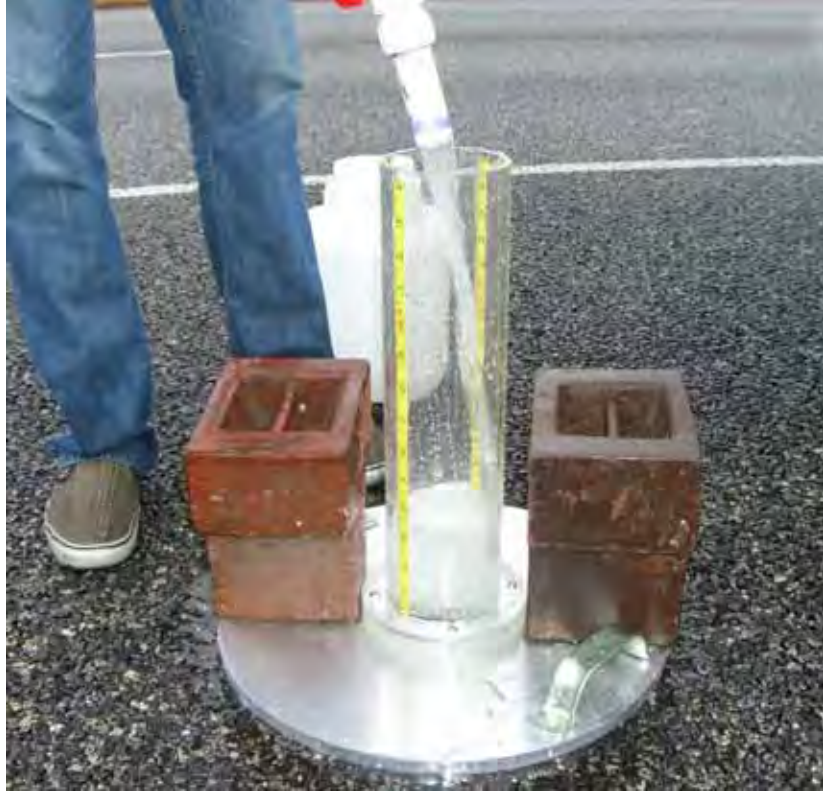
Figure 6-5 Constant Head Test
