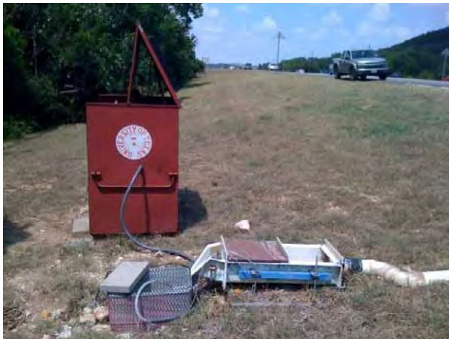
Figure 2-6: Flume and Sampling Box at Loop 360
