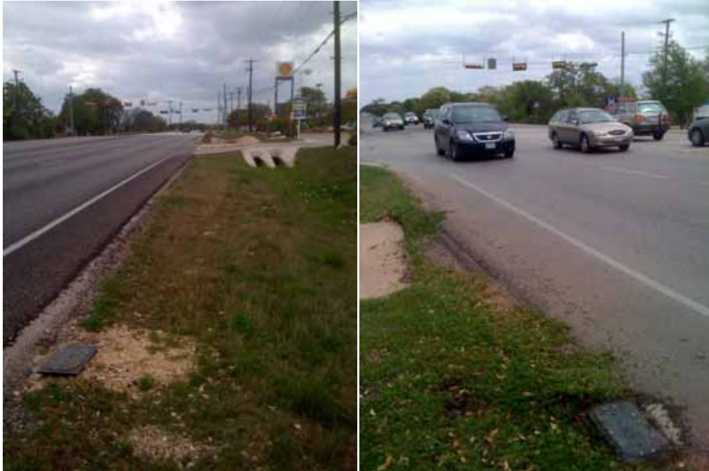
Figure 2-8: Passive Samplers at RR 620, PFC (Left) and Conventional Pavement (Right)
