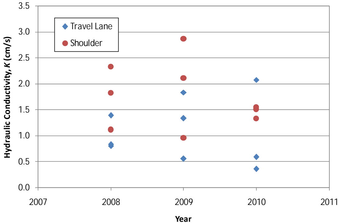
Figure 3-62: Travel lane versus shoulder hydraulic conductivity data on Loop 360
