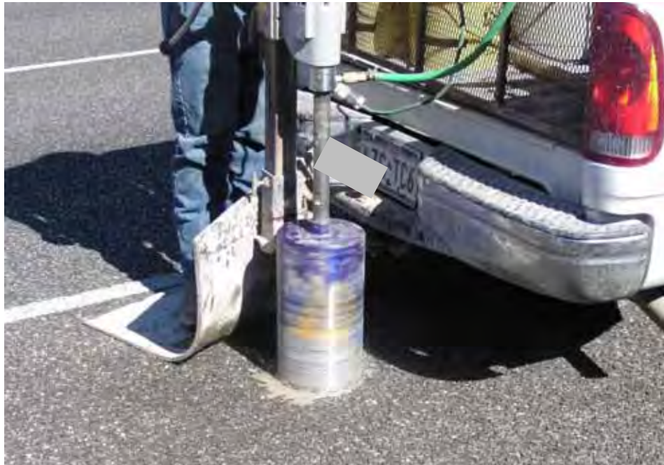
Figure 3-4: Drill press used for core extraction
