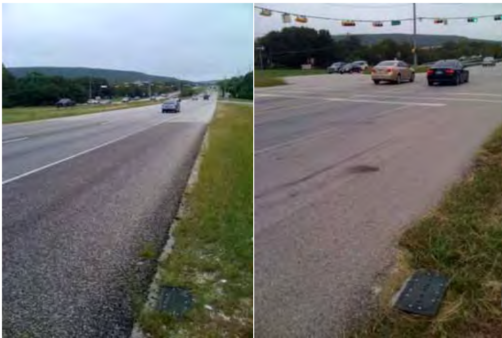
Figure 2-7: Passive Samplers at Loop 360, PFC (Left) and Conventional Pavement (Right)
