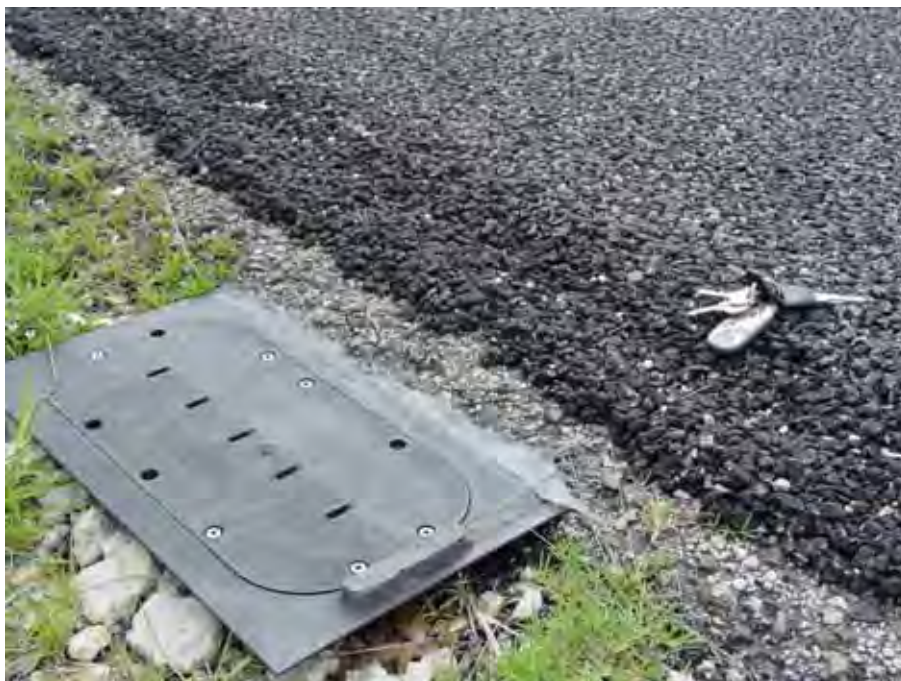
Figure 2-3 Photograph of installed sampler at edge of pavement.
