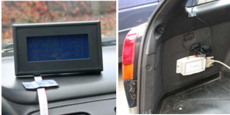
Figure 3.1: On-board mileage-counting equipment in the Oregon Pilot Project
