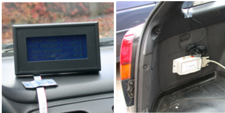
Figure 2.6: On-board mileage-counting equipment in the Oregon Pilot Project
