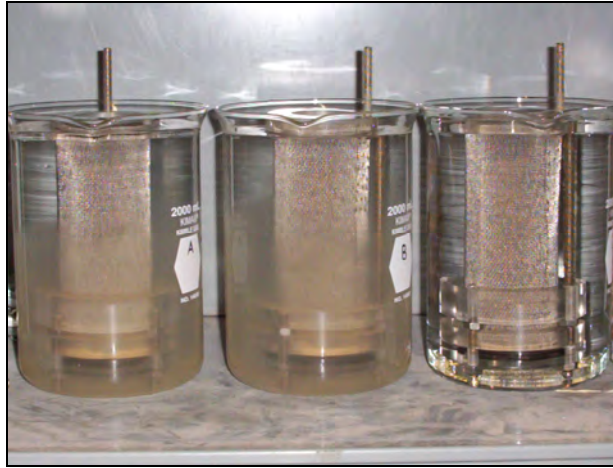
Figure 4.8: Submerged specimens during the wetting portion of cyclic wetting and drying test series.
