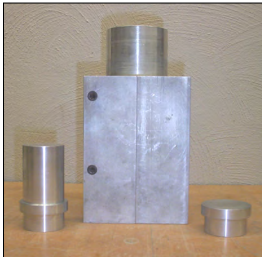
Figure 4.2: Assembled mold with bases used to produce 3-inch and 5-inch specimens.
