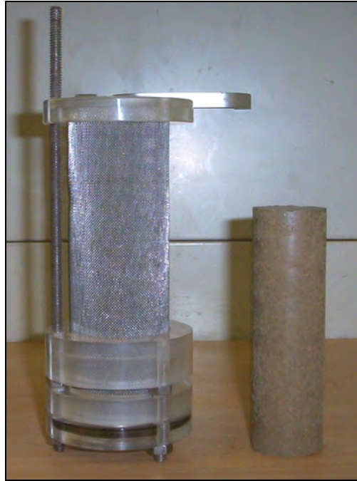
Figure 4.7: Cyclic wetting and drying specimen holder and compacted specimen.
