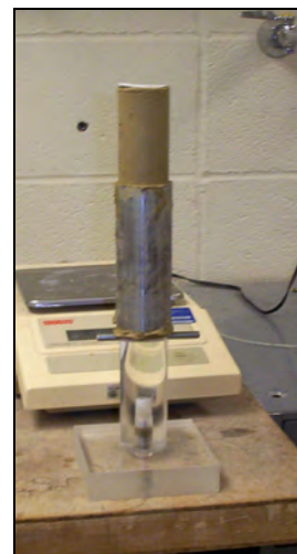
Figure 4.12: Trimmed and extruded specimen.
