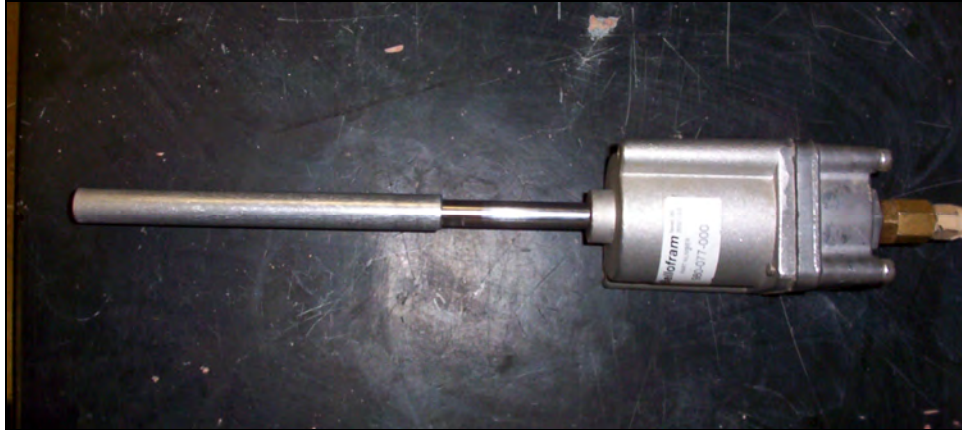
Figure 4.3: Marsh-Bellofram actuator air piston with aluminum rod.
