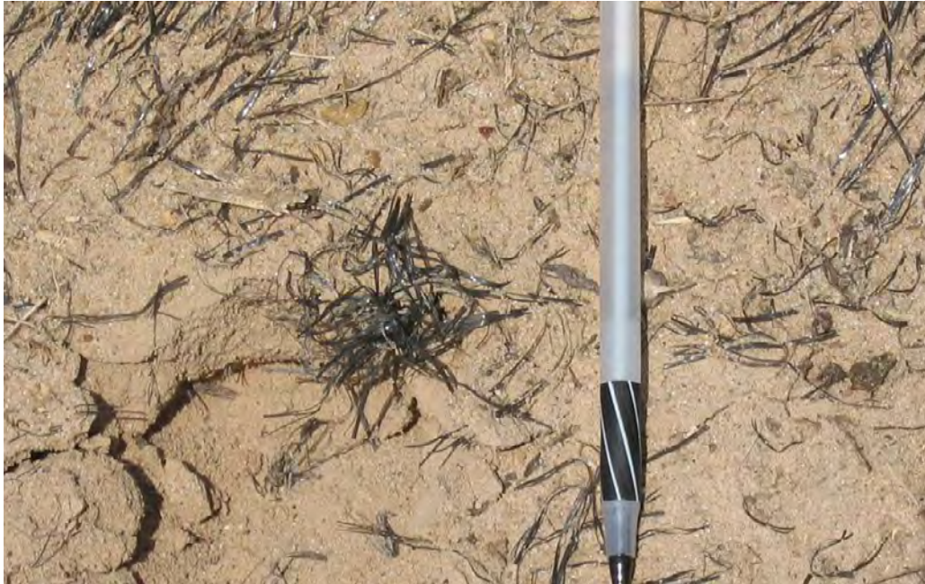
Figure D.52 Fibrillated Polypropylene Fibers Located at Embankment Surface.
