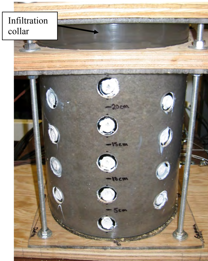
Figure 4.18: Infiltration setup for Soil Column 3
