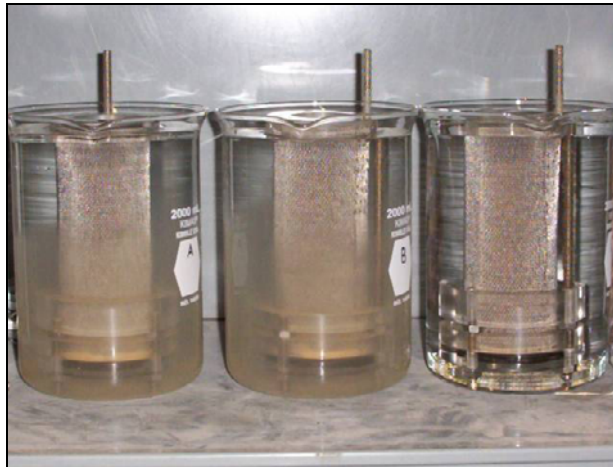
Figure 5.2: Submerged specimens during the wetting portion of cyclic wetting and drying test series
