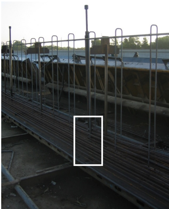
Figure 3.10 Typical Deflected Strands at Precast Plant D (Photographs courtesy of David Birrcher)
