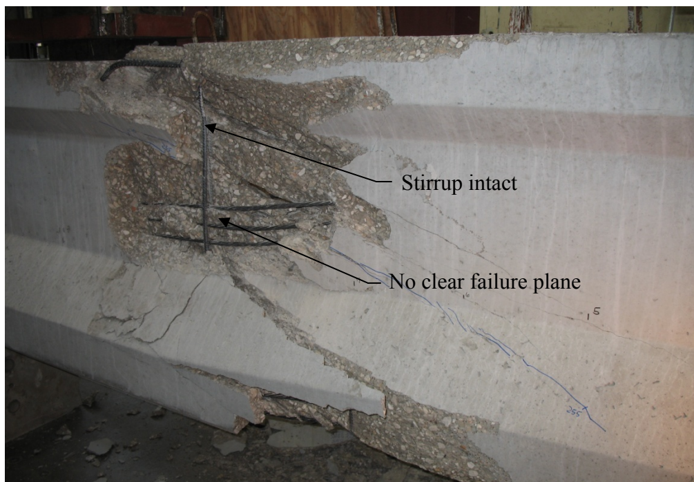
Figure 5.10 Web Crushing Failure
