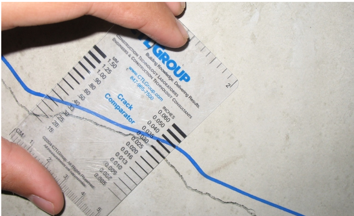
Figure 4.9 Measurement of Diagonal Crack Width
