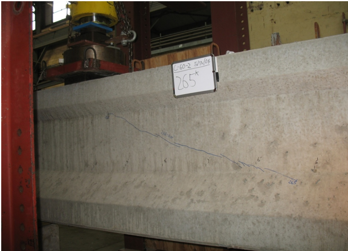
Figure 5.4 First Web-Shear Crack on Beam CD-60-2
