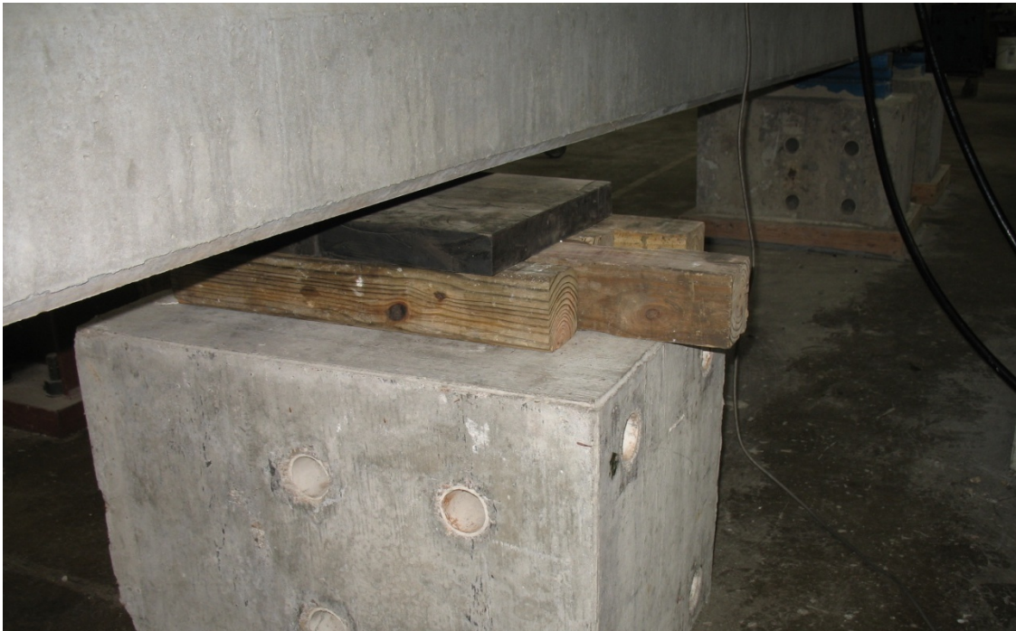
Figure 5.11 Stopper Block used to Catch Beam after Failure
