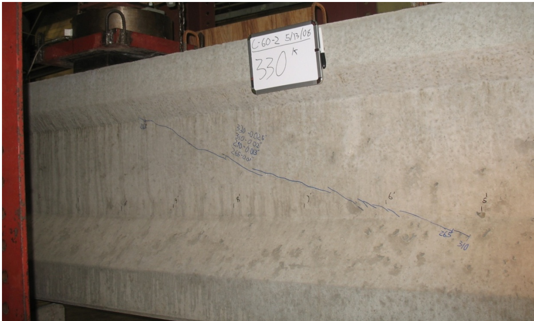
Figure 5.5 Last Load Stage on Beam CD-60-2
