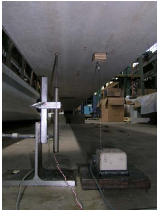
Figure 4-13: Midspan deflection instruments used in static testing of full-scale beams
