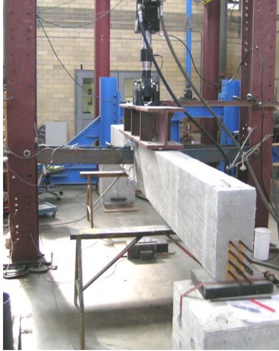
Figure 4-17: Picture of test setup for fatigue testing
