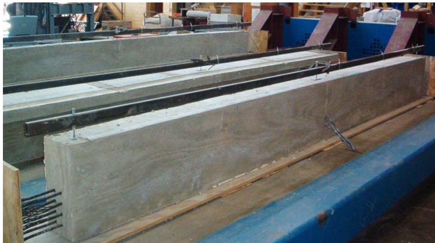
Figure 6-8: Picture of initial camber setup (photograph courtesy of Alfredo Castro)
