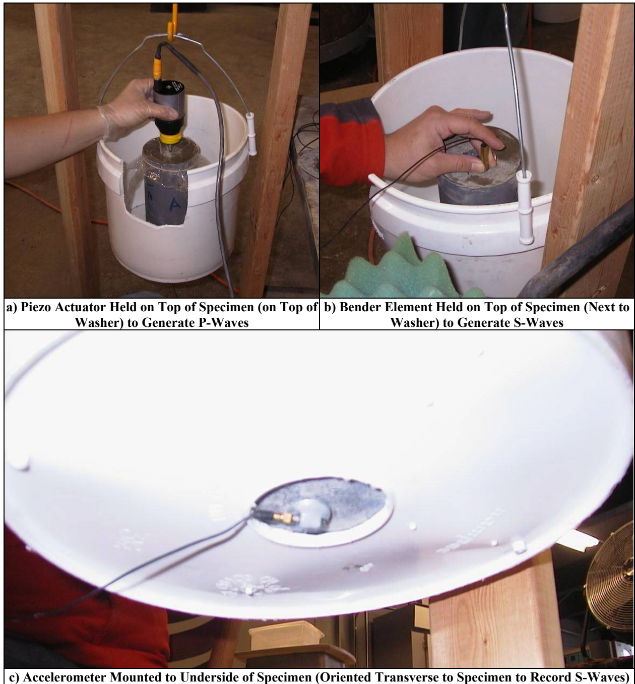
Figure 5.23 Specimen Suspended in Hanging Bucket for Testing
