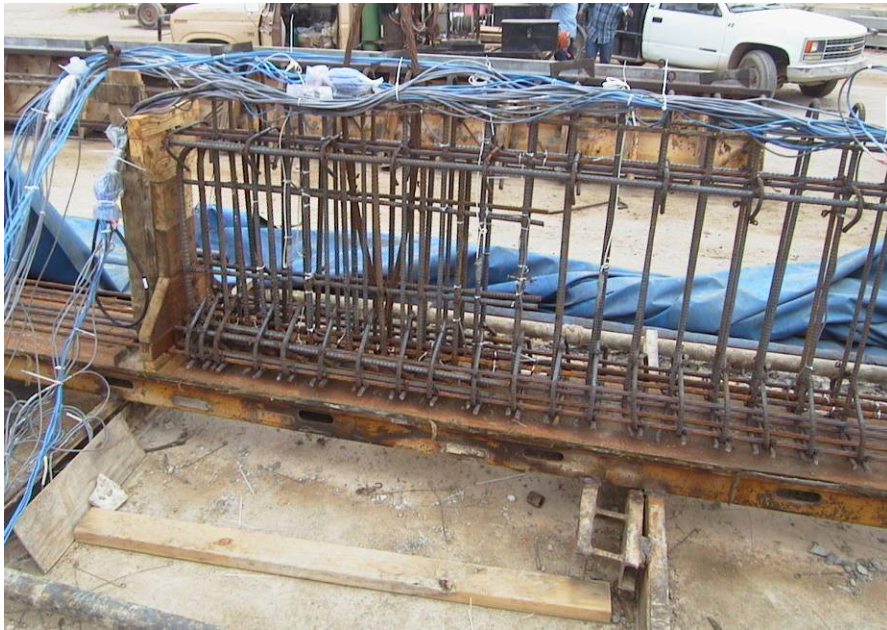
Figure 9.2 Reinforcement in Type A Beams
