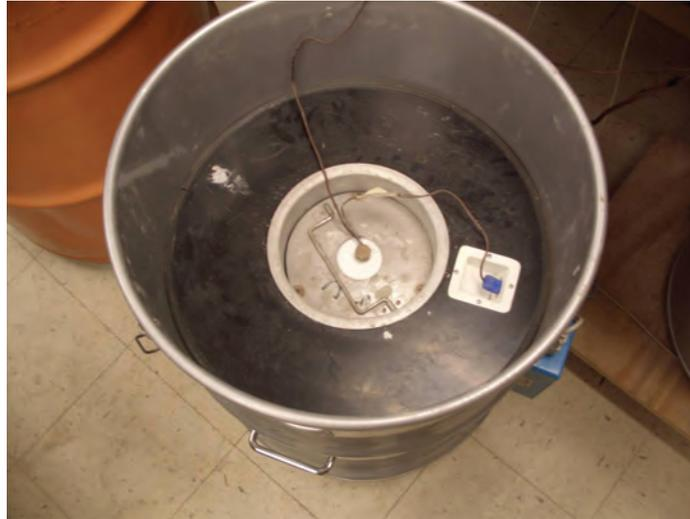
*Figure 5.1 Semi-adiabatic calorimeter*
