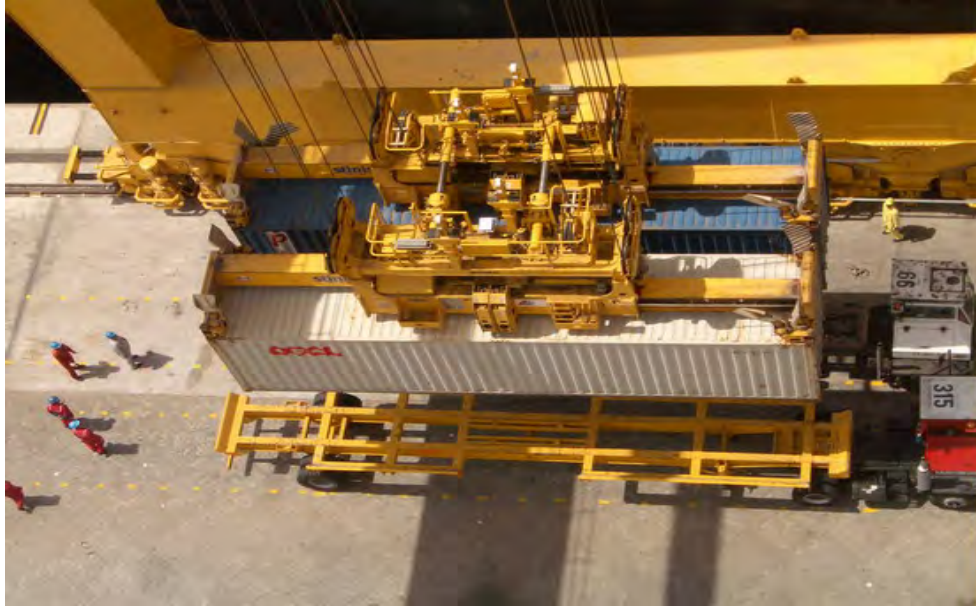
Figure B.2: Crane with twin 40' lift capacity unloading containers at the Port of Dubai Source: Shanghai Zhenhua Port Machinery Co.
