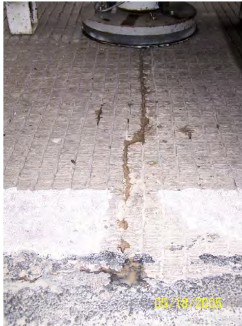
Figure 3.15 Pumping effect caused by FWD testing in a crack
