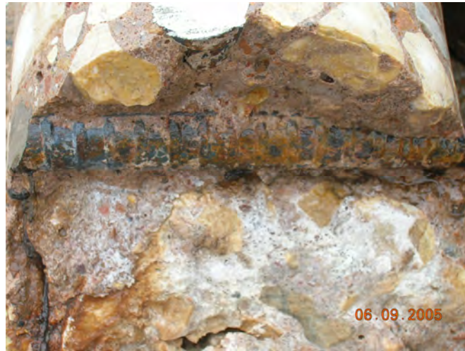
Figure 3.24 Detail of old concrete deterioration in one of the core samples
