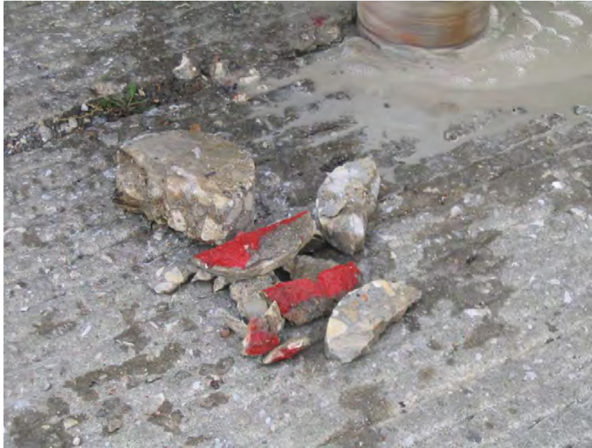
Figure 3.9 Delaminated portion of BCO in a core sample broken during drilling operation
