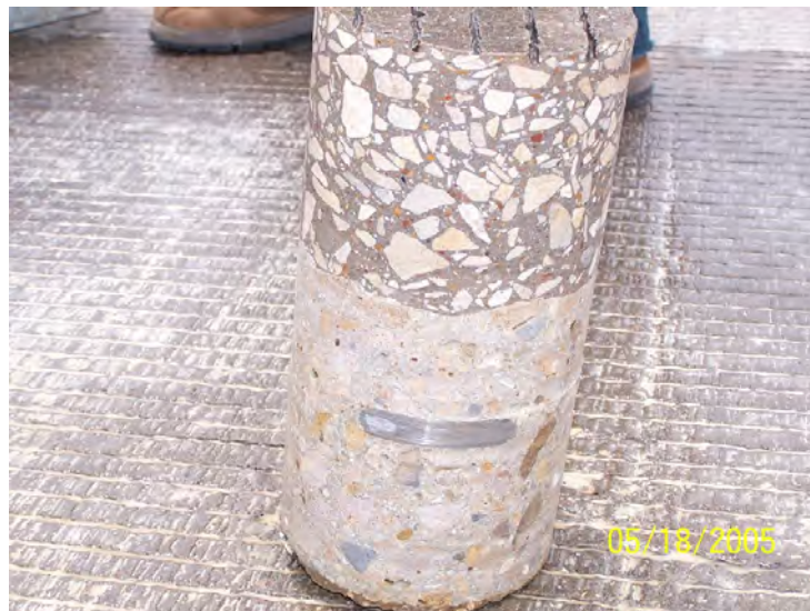
Figure 3.11 Core obtained from IH 30 in Fort Worth
