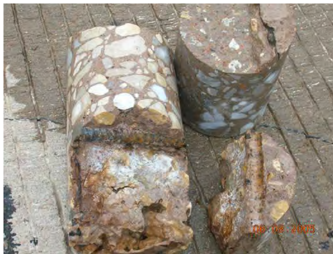
Figure 3.23 Old concrete deterioration in one of the cores
