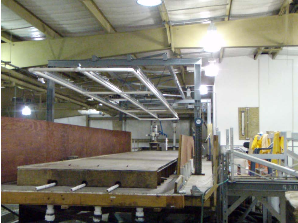
Figure 3.2: Picture of physical model viewed from downstream end showing rainfall simulator, three sample ports located near end of model surface, and inclined manometer board located to the right side of the surface platform
