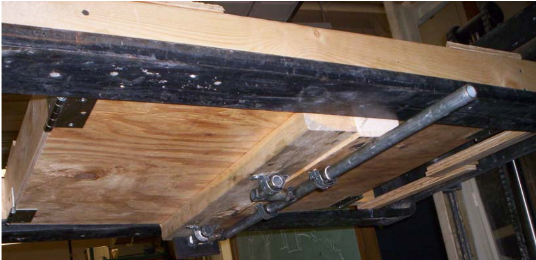
Figure 4.19: Drop Test Release Mechanism
