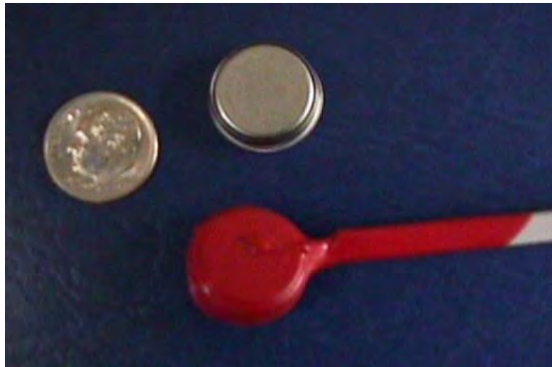
Figure 4.1 Dallas Semiconductor Thermochron i-Button
