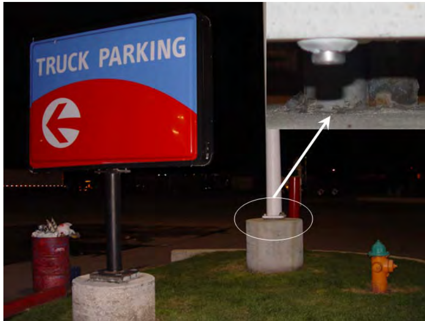
Figure 4.9 Amarillo ambient sensor hidden under base of sign (inset is close-up of circled area)
