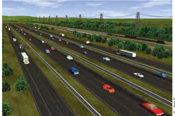
Figure 1.2. Conceptualized Layout of Separated Lanes for Cars, Trucks, Rail and Utilities
