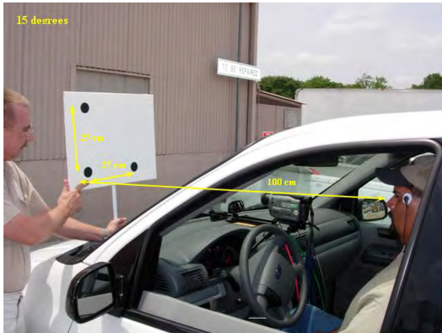
Figure 4.7 Eye Movement Angular Calibration for 15 Degree Marks
