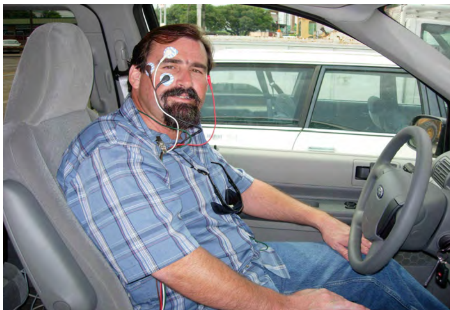
Figure 4.6 The Position of EOG Electrodes on Driver's Face
