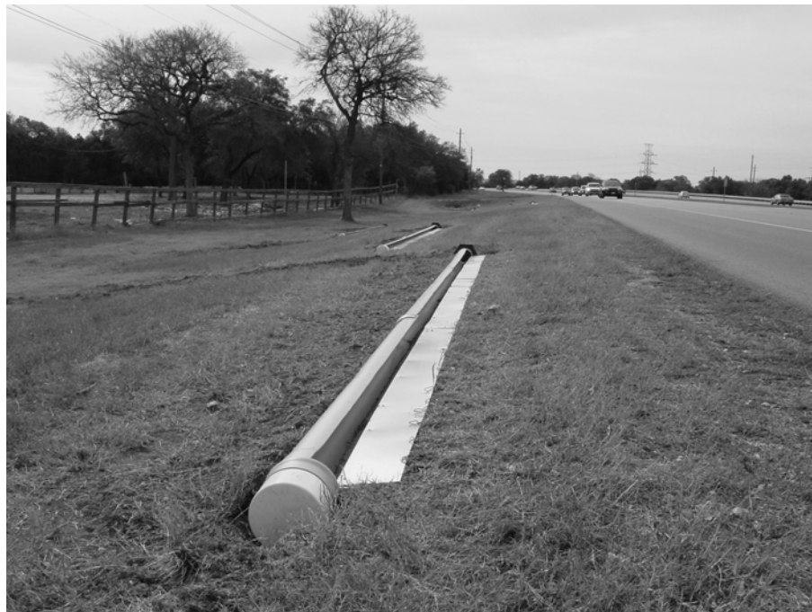
Figure 4.12 Photograph of installed collection pipe at Austin Site 2
