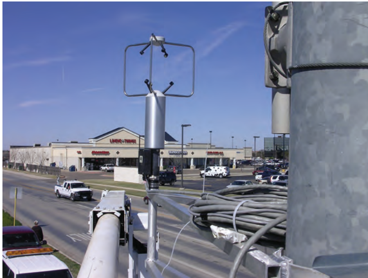
Figure 4.7: Ultrasonic anemometer attached to the pole
