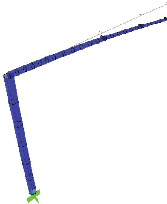
Figure 4.15: Deflected shape of finite element model of signal structure
