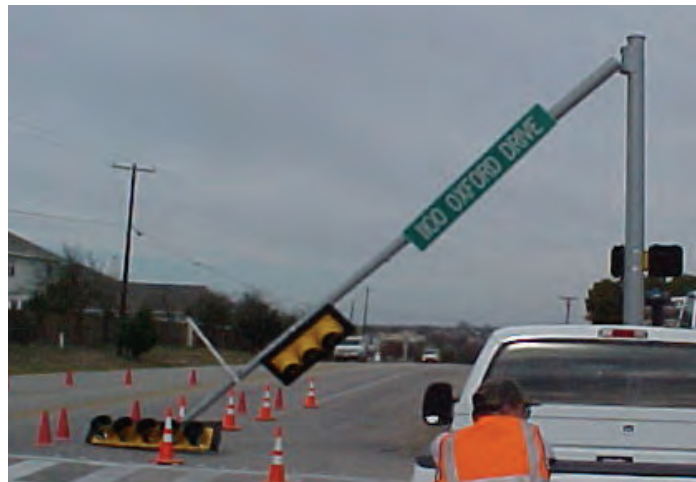
Figure 1.1: Failure of traffic signal structure in Pflugerville
