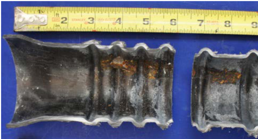
Figure 5.19 – Mild Staining of Plastic Duct
