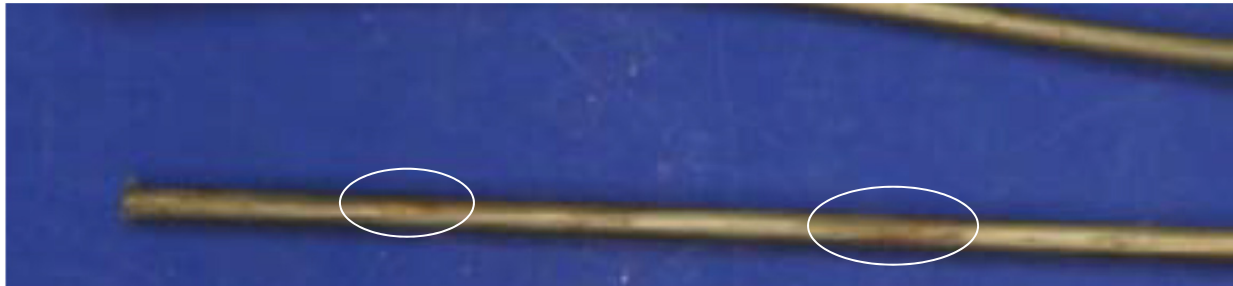
Figure 5.26 – Highlighted Mild Discoloration on Interior of Flow-Filled Strand
