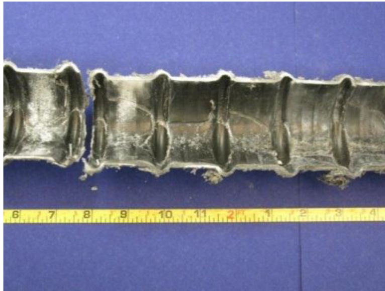
Figure 5.17 – Damage Caused by Stainless Steel Strand
