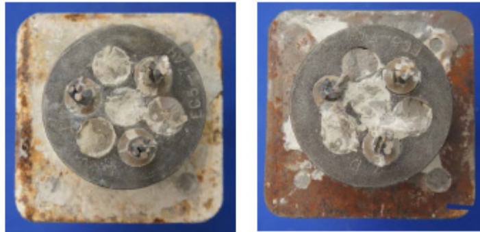
Figure 5.29 – Corrosion on Exposed Faces of Galvanized (left) and Non-Galvanized (right) Anchorage Plates
