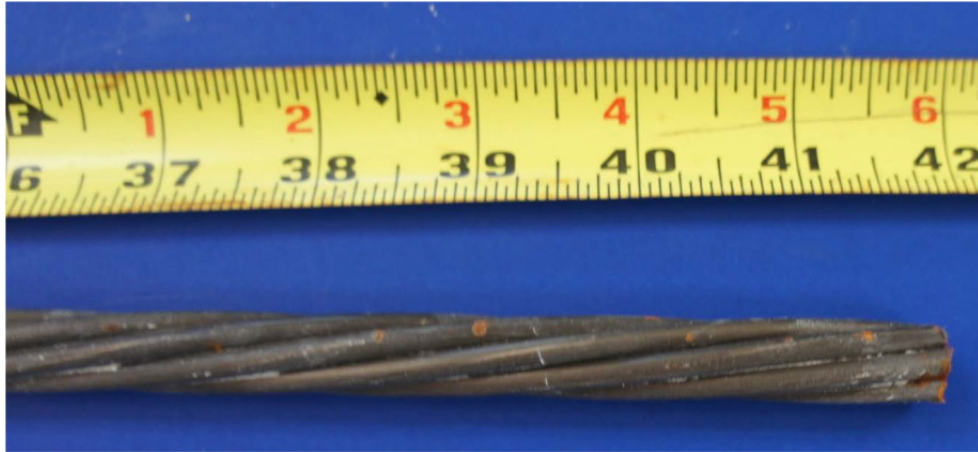
Figure 5.27 – Discoloration on Conventional Strand
