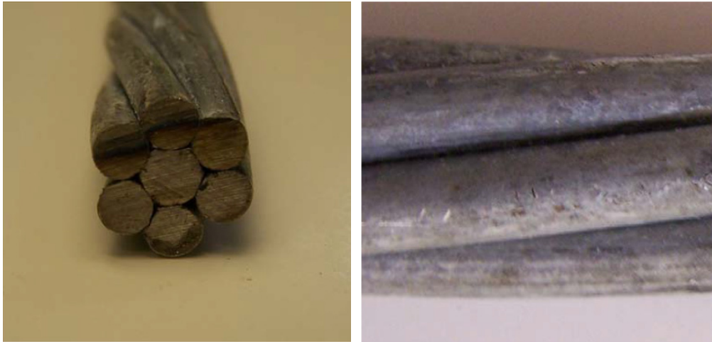
Figure 2.6 – Hot-Dip Galvanized Strand Cross Section and Exterior
