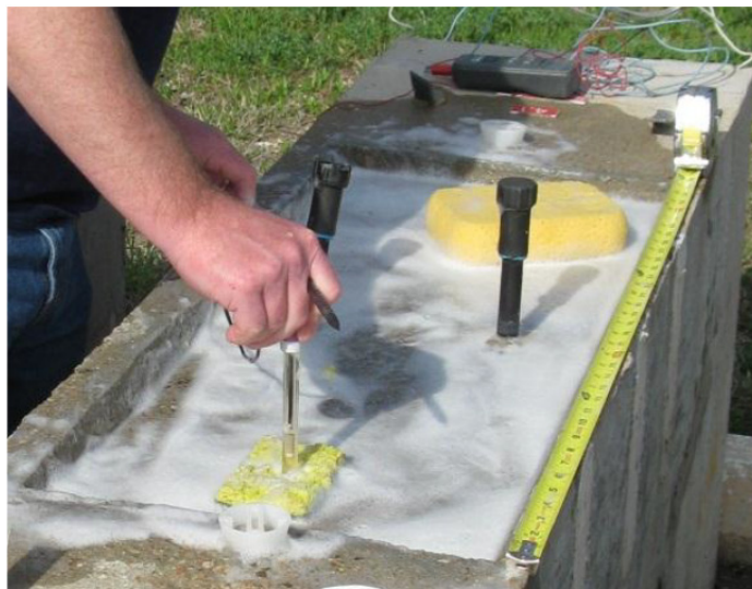
Figure 4.1 – Half-Cell Testing in Ponding Region
