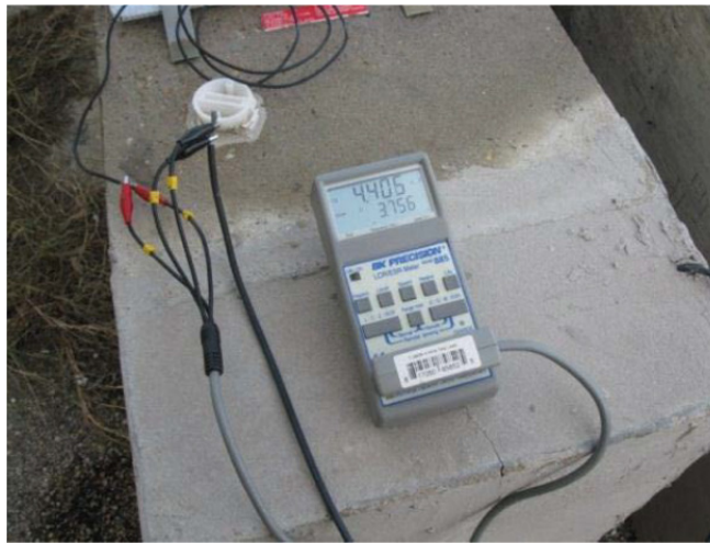
Figure 4.2 – AC Impedance Testing Meter
