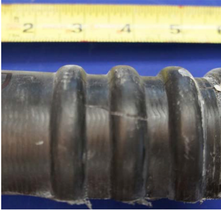
Figure 5.18 – Crack in Specimen 7.2
