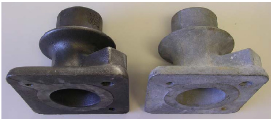
Figure 2.17 – Non-Galvanized Anchorage (left) and Hot-Dip Galvanized Anchorage (right)
