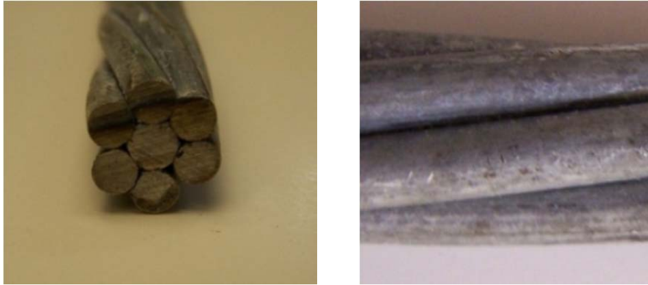
Figure 1.6: 0.5 in. Hot Dip Galvanized Strand
