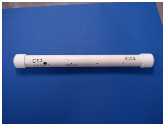
Figure 3.2: Pipe Configuration with Capped Ends and Holes Drilled
