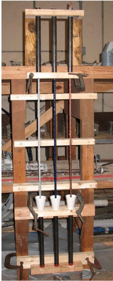
Figure 2.1: Setup Used to Cast Ends onto the Strands
