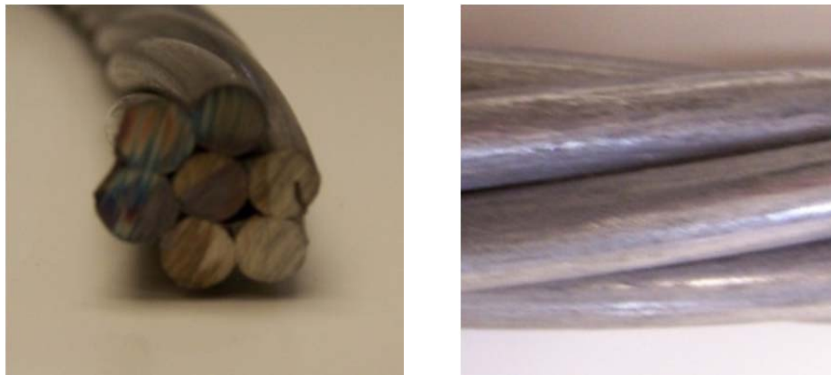
Figure 1.7: 0.6 in. Stainless Steel Strand
