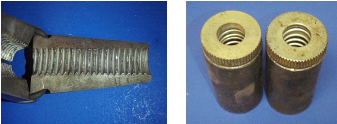
Figure 4.11: Chucks Used to Damage Epoxy Coating
