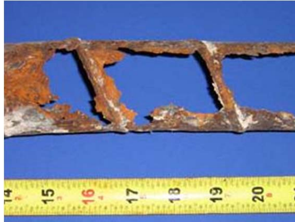
Figure 1.3: Corroded Hot Dip Galvanized Duct
