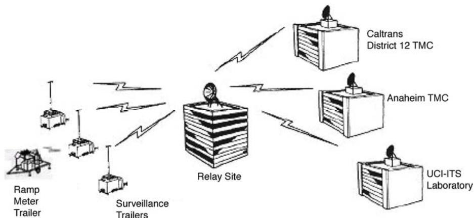
Figure 3-1. Transmission of video and data among trailers, relay site, TMCs, and UCI during the mobile surveillance and wireless communication systems field operational test (Klein, 1999).
