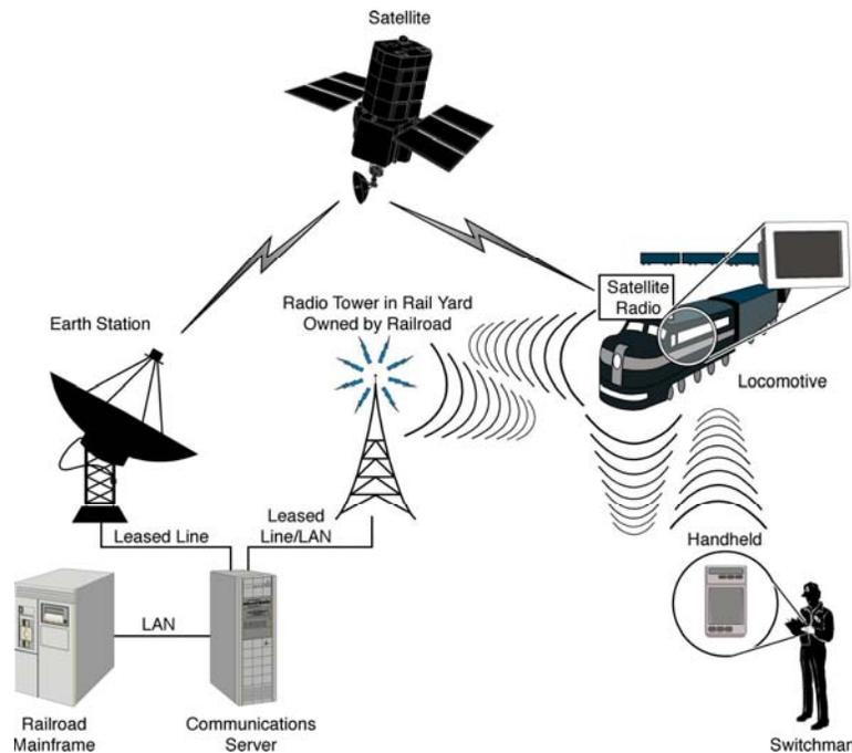
Figure 2-4. Communication technology used in commercial vehicle operation – an example in railroad management (SAIC, 2002).
