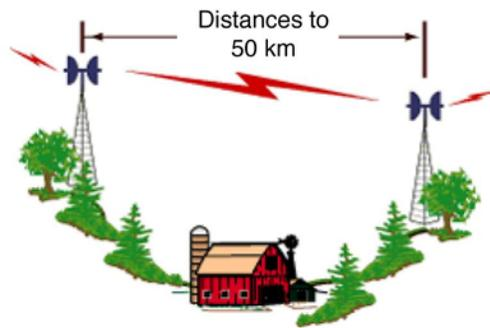
*Figure 3-2. Maximum distance between base stations for fixed wireless technology (Rysavy, 2002).*
