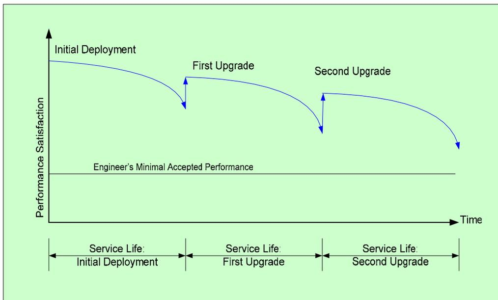
Figure 4-4. Example of lifetime of a wireless technology alternative.
