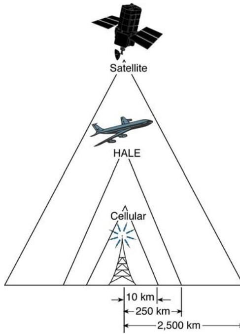
Figure 3-3. Service range of three types of wireless communication technologies (Rysavy, 2002).
