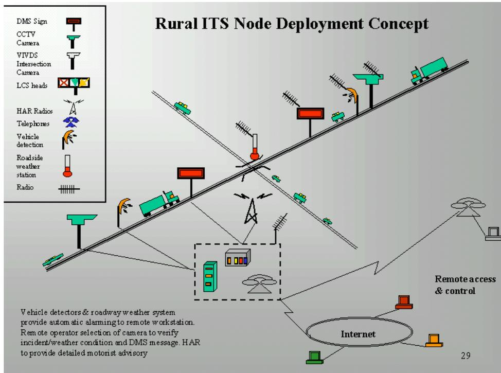
Figure 2-3. Rural ITS node deployment concept.
