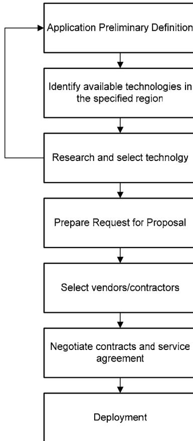
Figure 4-1. Wireless technology acquisition project process.
