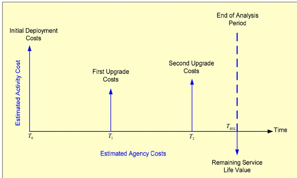
Figure 4-5. Expenditure diagram with activity, costs, and timing shown.
