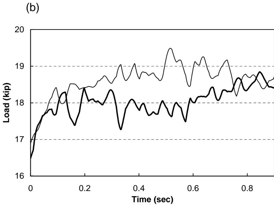
Figure 3.2. Load time histories on (a) front- and (b) rear-axle tires with vehicle speed of 20 mph
