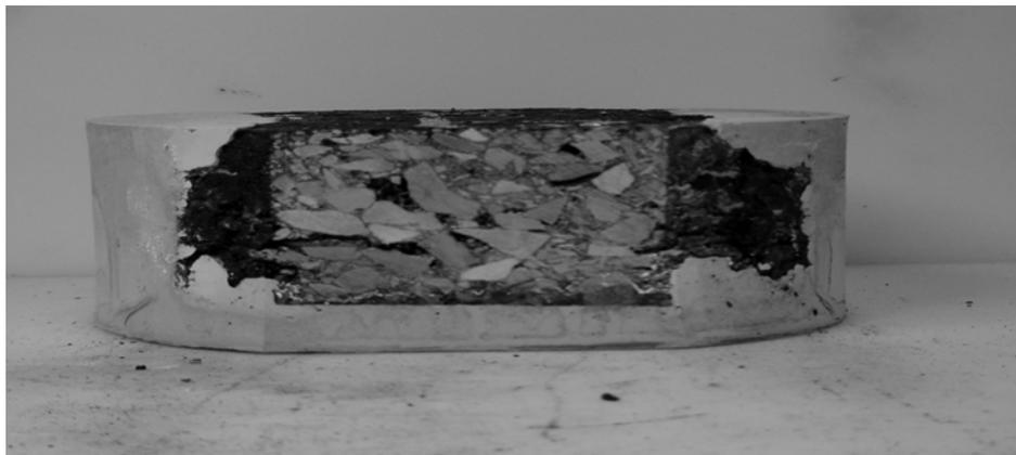
*Figure 6.7 Gypsum repaired Hamburg specimen*
