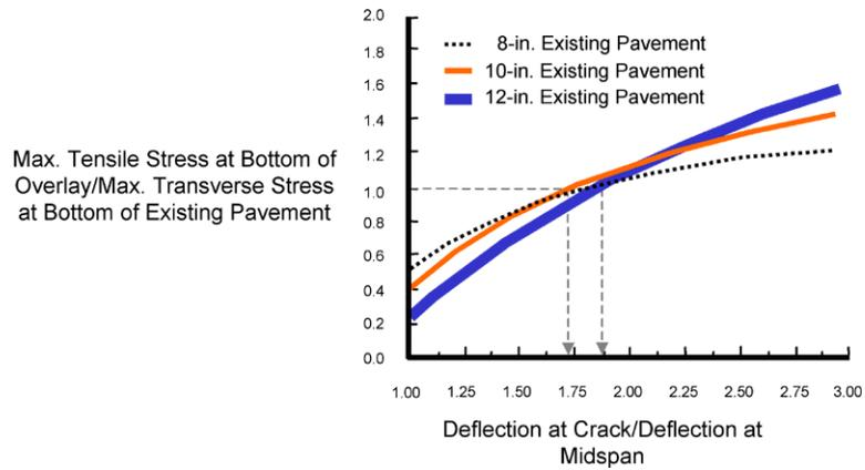
*Figure 5.3 Stress ratio versus deflection ratio for low-modulus overlay concrete as criterion for BCO selection*
