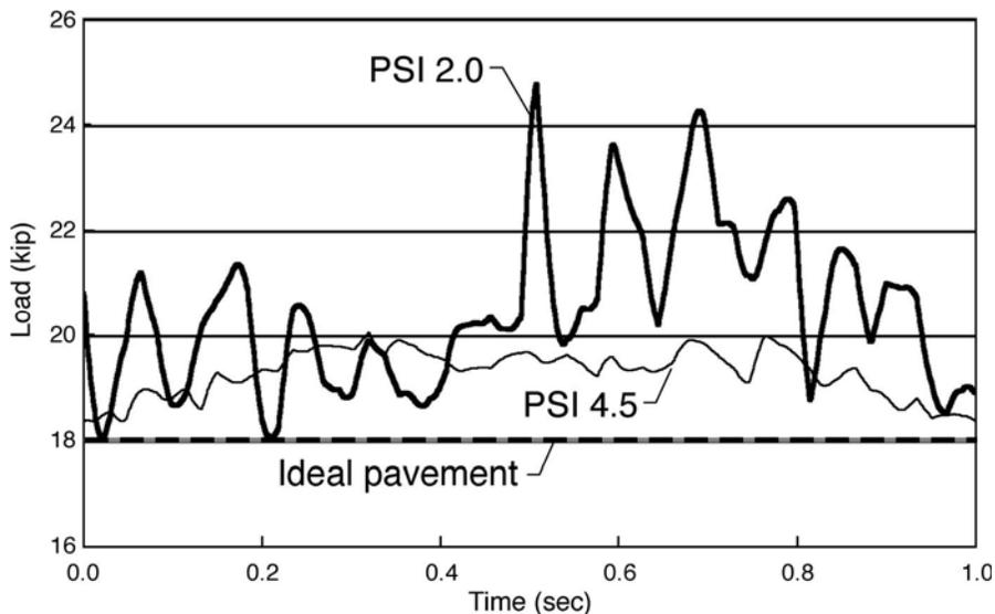
Figure 3.12. Load time histories on front-axle tires for different surface profiles
