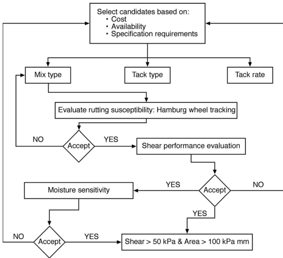
Figure 6.22. Decision tree for AC mix and tack coat selection
