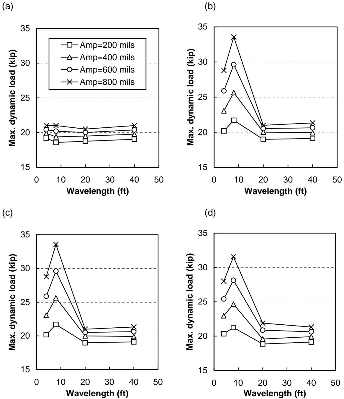
Figure 3.9. Effect of roughness wavelength on dynamic loading for a vehicle speed of (a) 20, (b) 40, (c) 60, and (d) 80 mph
