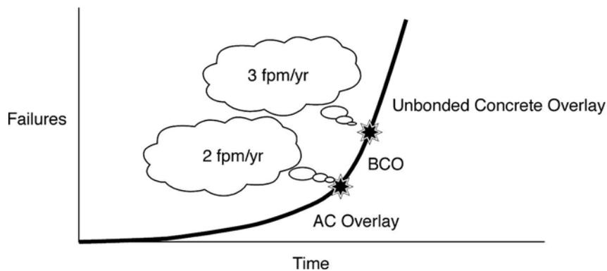
*Figure 4.9 Decision criteria for AC overlays, BCOs and unbonded concrete overlays based on failure rate*
