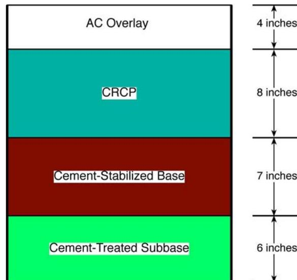
*Figure 5.5 Cross sectional view of the IH-20 structure in Harrison Co.*
