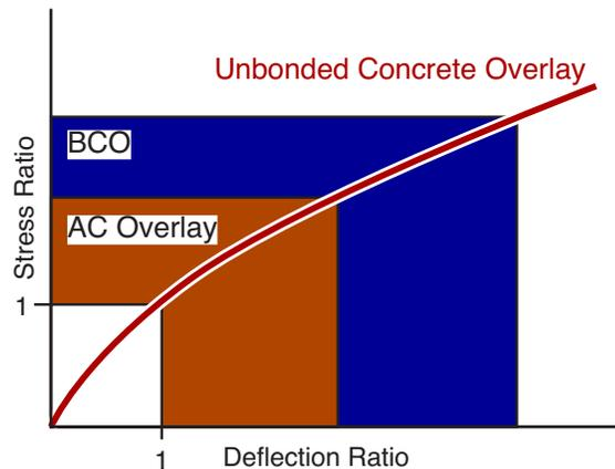
*Figure 5.2 Applicability of different types of overlay according to a deflection criterion*
