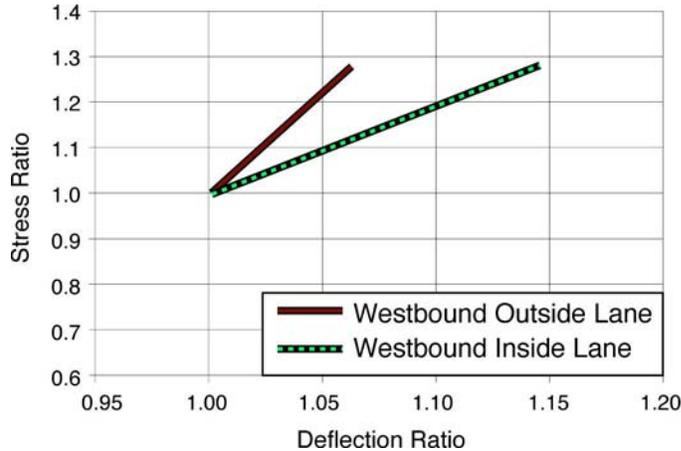
*Figure 5.6 Stress and deflection ratios for IH-20 section near Marshall*
