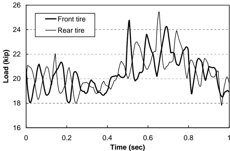
Figure 3.13. Load time histories on front- and rear-axle tires on PSI 2.0 pavement
