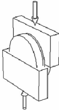
*Figure 6.2 Direct shear testing configuration*
