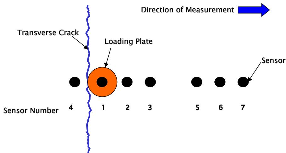
Figure 5.1 FWD downside loading and sensor arrangement for deflection at crack measurement (plan view)
