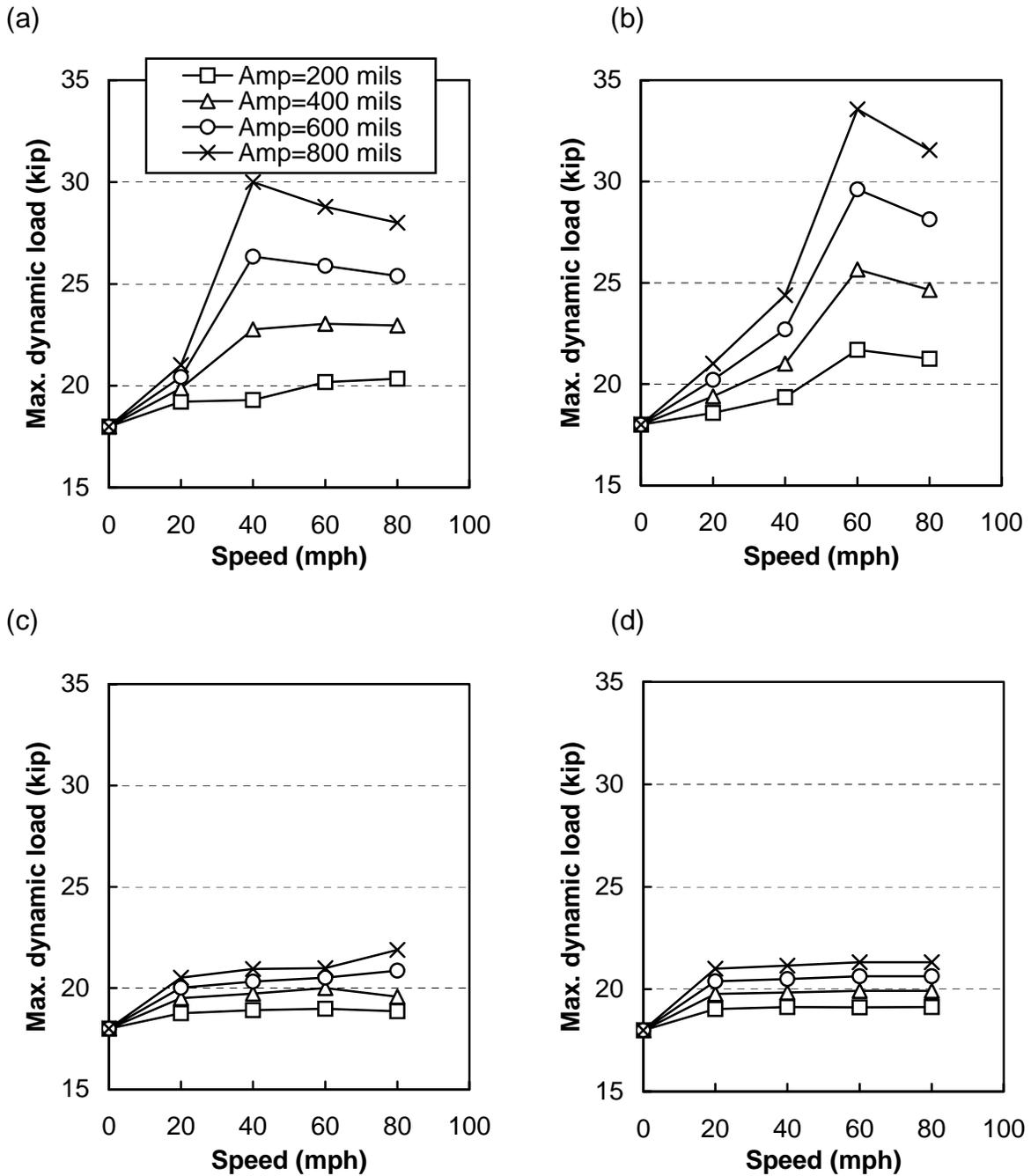
Figure 3.11. Effect of vehicle speed on dynamic loading for a roughness wavelength of (a) 4, (b) 8, (c) 20, and (d) 40 ft
