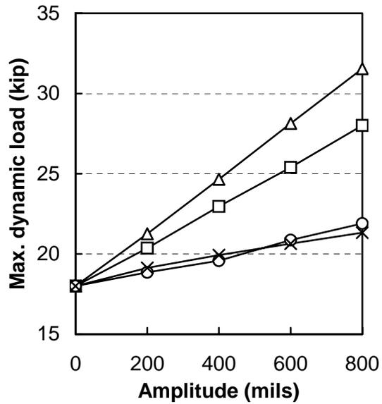
Figure 3.6. Effect of roughness amplitude on dynamic loading for a vehicle speed of (a) 20, (b) 40, (c) 60, and (d) 80 mph
