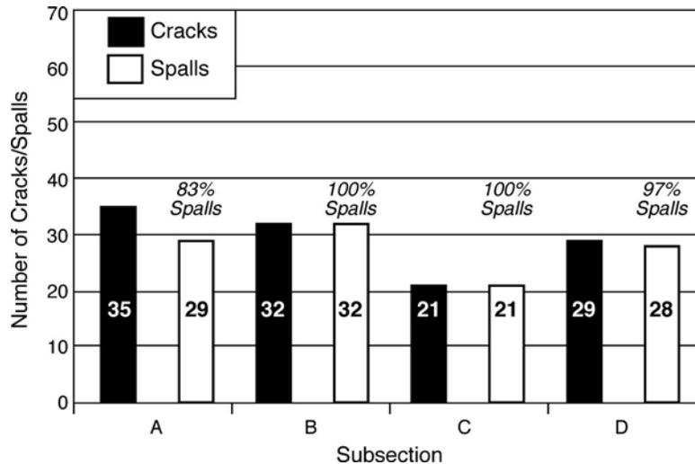
Figure 4.6 Crack spalling on SH6 winter sections (SRG)
