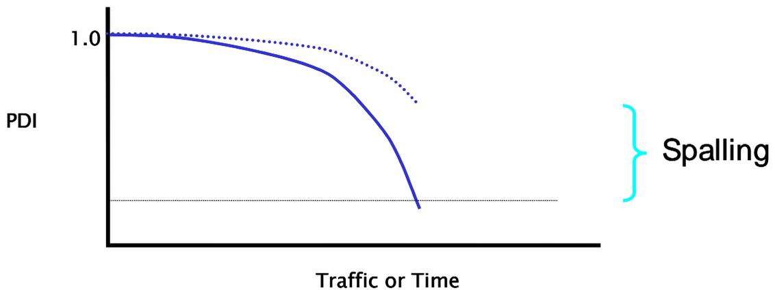
Figure 4.3 Inclusion of spalls in the PDI equation
