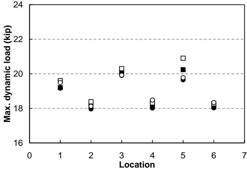
Figure 3.17. Dynamic loads on the pavements on IH-20 (a) before and (b) after new overlays
