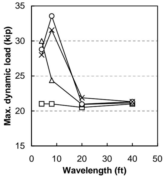
Figure 3.8. Effect of roughness wavelength on dynamic loading for a roughness amplitude of (a) 200, (b) 400, (c) 600, and (d) 800 mils
