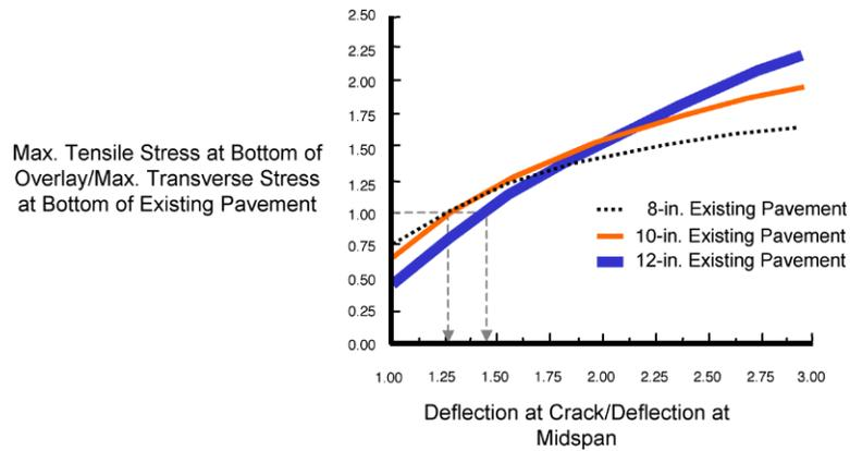
*Figure 5.4 Stress ratio versus deflection ratio for high-modulus overlay concrete as criterion for BCO selection*
