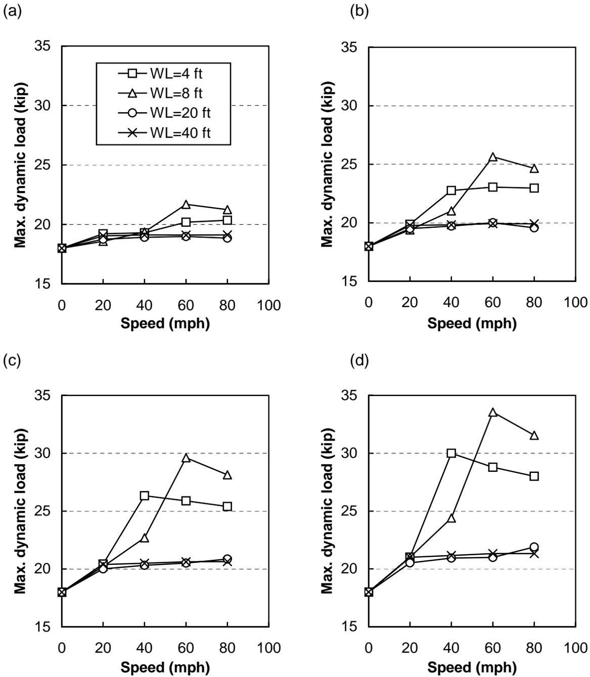
Figure 3.10. Effect of vehicle speed on dynamic loading for a roughness amplitude of (a) 200, (b) 400, (c) 600, and (d) 800 mils
