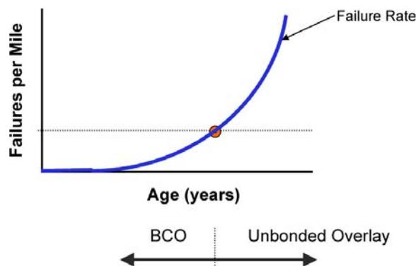
*Figure 4.7 Performance curve based on rate of failures per mile per year as criterion for bonded or unbonded overlays*
