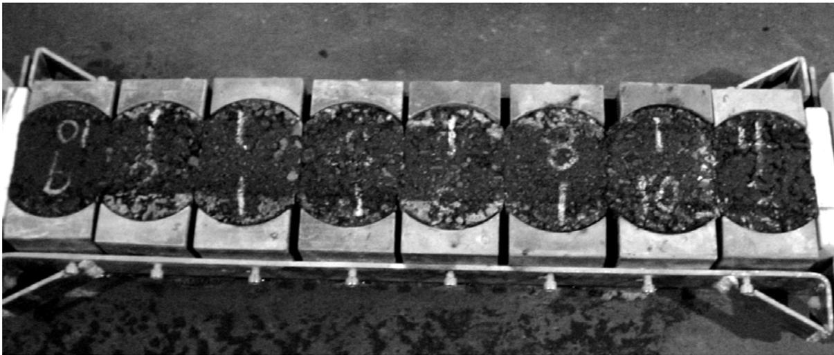
*Figure 6.6 MMLS3 test configuration*
