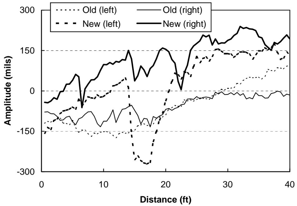
Figure 3.1. Typical surface profile data collected on IH-20 on old and new AC overlays placed over a CRCP
