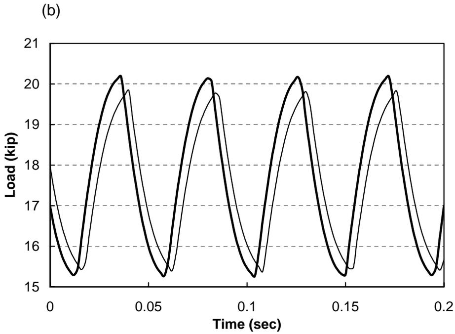
Figure 3.5. Load time histories on front- and rear-axle tires when vehicle speed is (a) 20 and (b) 60 mph
