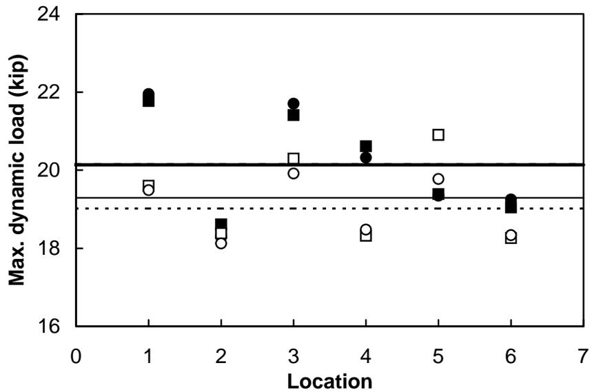
Figure 3.18. Comparison of dynamic loads on the pavements on IH-20 for a vehicle speed of (a) 20 and (b) 60 mph
