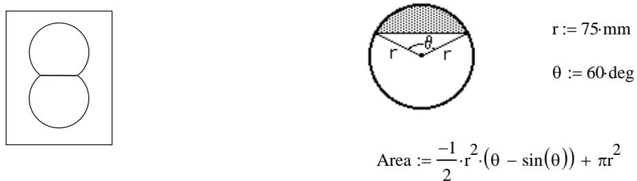
Figure 6.1 Specimen configuration for Hamburg testing and associated surface area calculations
