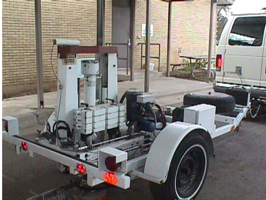
Figure 5.4 Falling weight deflectometer
