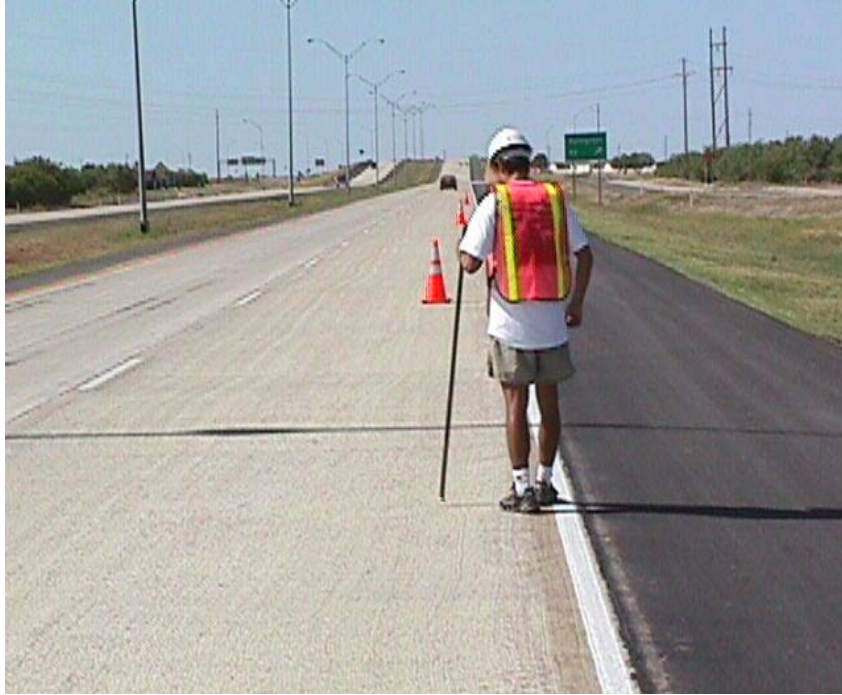
Figure 7.11 Sounding for delamination detection
