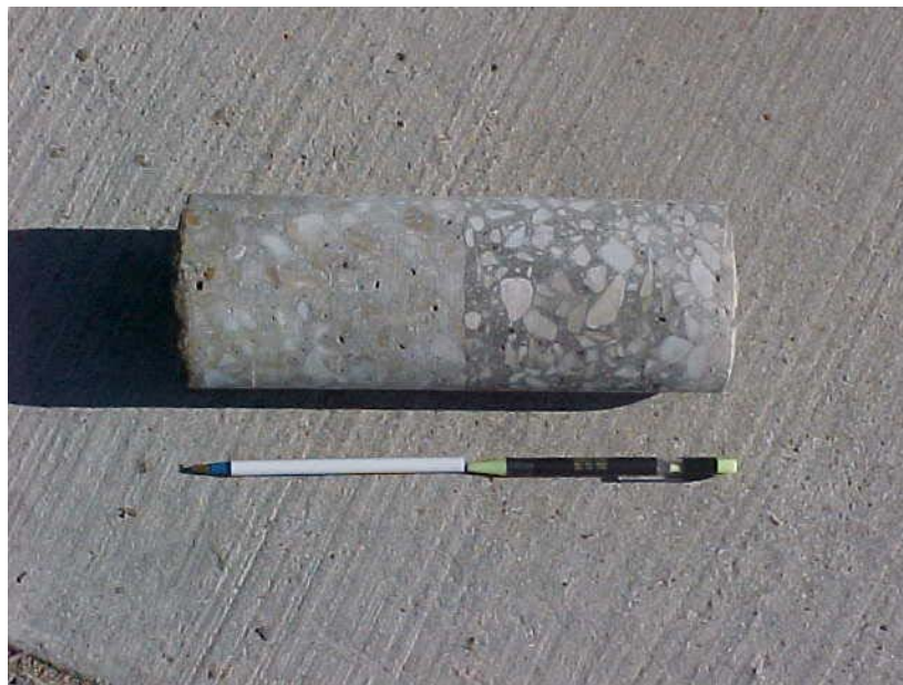
Figure 9.29 Eastbound core for petrographic testing
