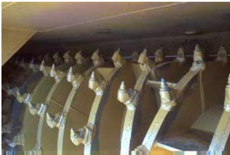
Figure 6.3 Rotomill tungsten carbide-tipped mandrel
