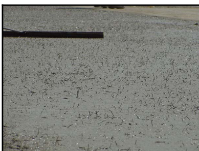
Figure 4 – Hairy Texture of Pavement Section Containing 6 pcy of SnF1
