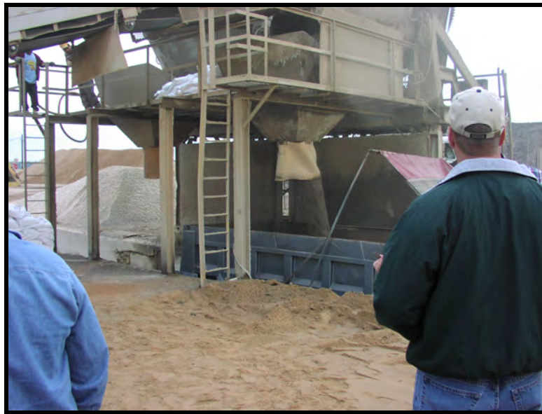
Figure 4.6: Manual Loading of Synthetic Fiber Bags into Concrete Mixer
