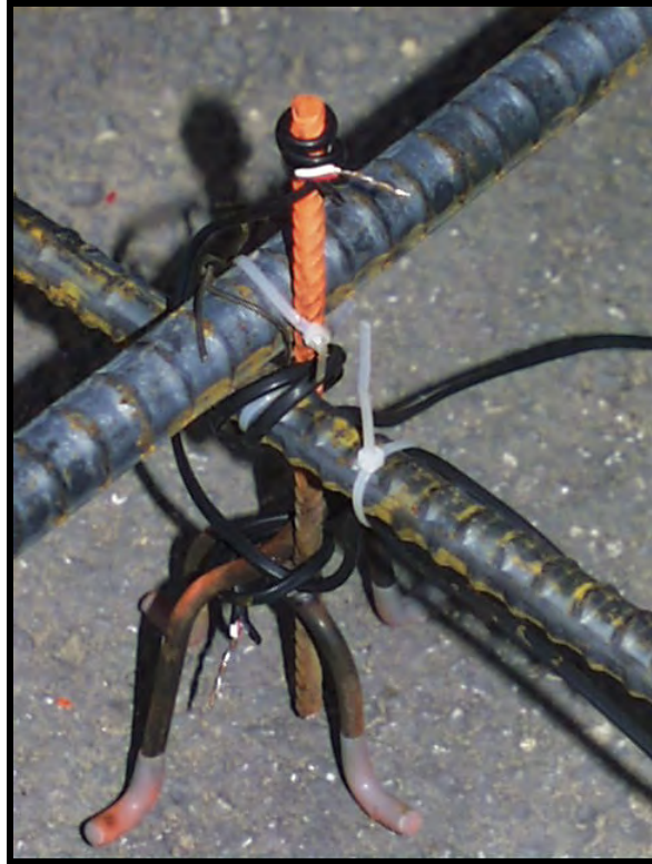
Figure 4.21: Close-up of Thermocouple Installation
