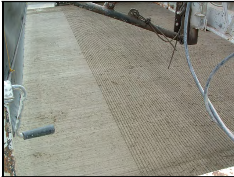
Figure 5.17: Fibers Disturbed during Tining (Section 2—SF1-25)
