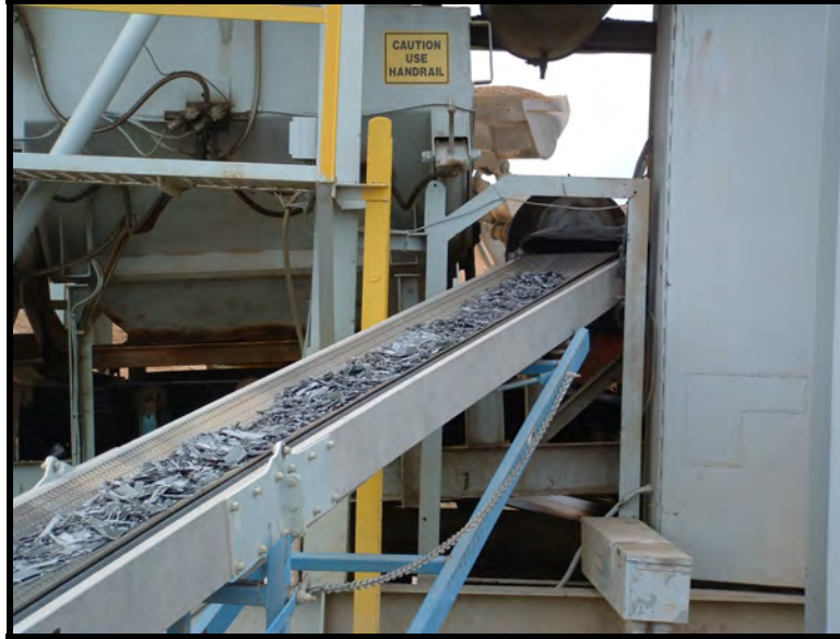
Figure 4.7: Conveyor Belt Loading of Steel Fibers into Concrete Mixer
