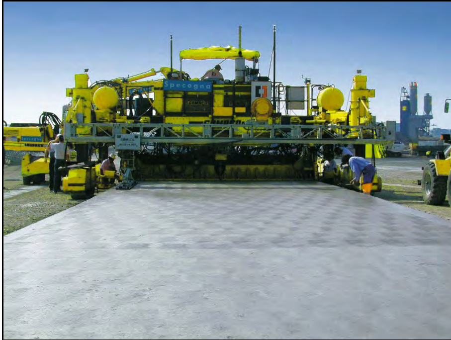
Figure 2.5: Slipform Paving Machine (Leica Geosystems 2002)
