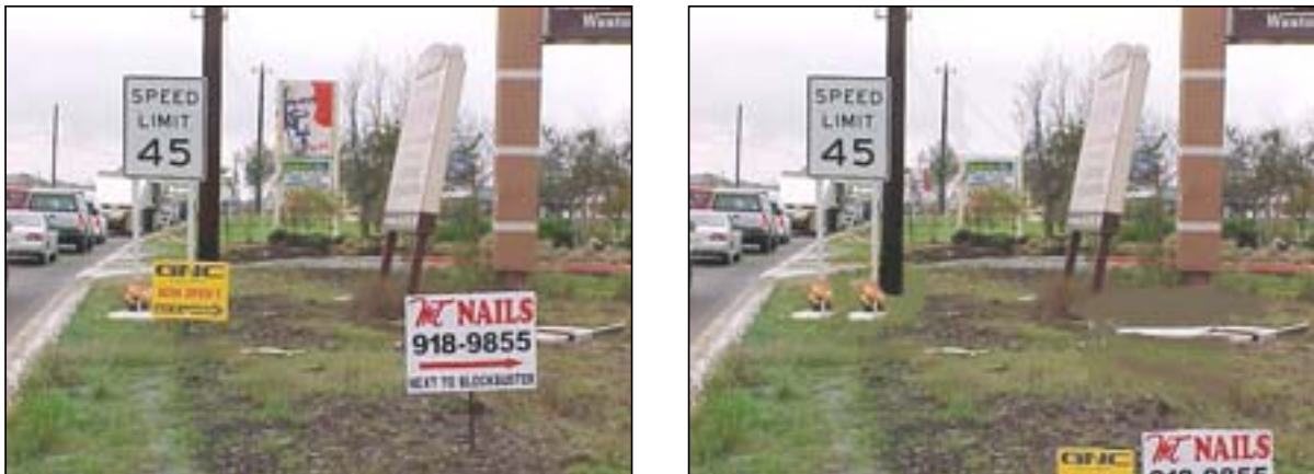
Figure 2.1 Relocation of commercial signs to ensure speed limit sign's dominance in the driver field of view (left, before relocating and right after relocating)
