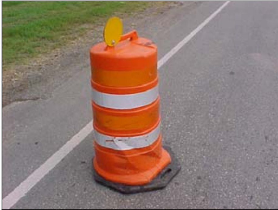
Photo C.3 Damaged plastic drum
