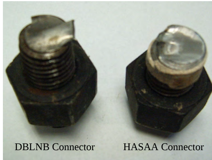
Figure 5.21: Failed sections of shear connectors
