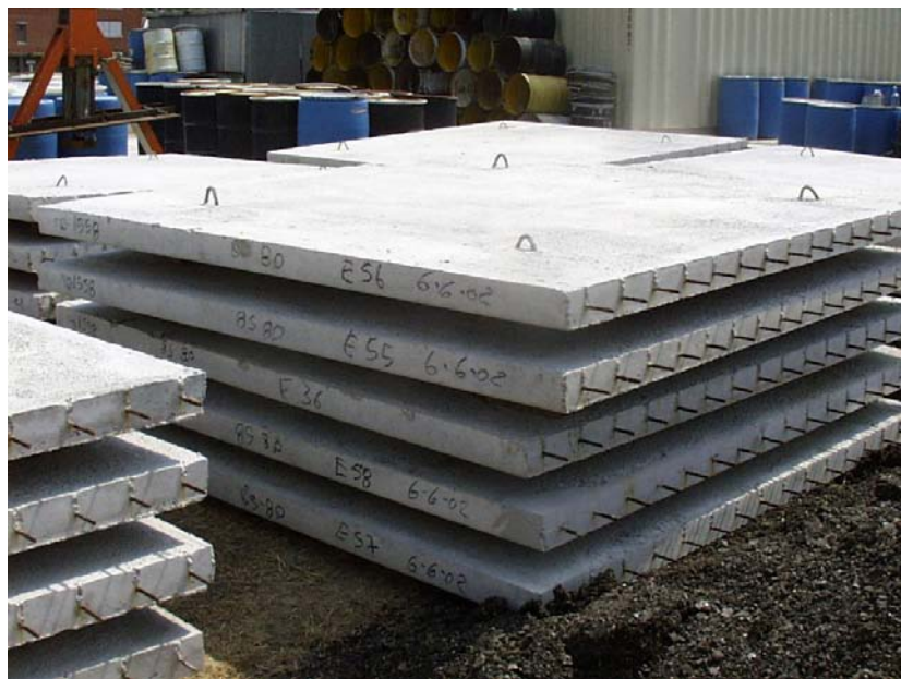
Figure 5.7 Photograph of actual PCP used in the construction of the LSBs
