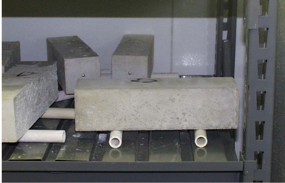
Figure 3.2 Free Shrinkage Prism (ASTM C157)
