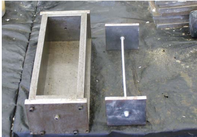
Figure 3.3 Mold and Restraining Cage for SCC Prism (ASTM C878)
