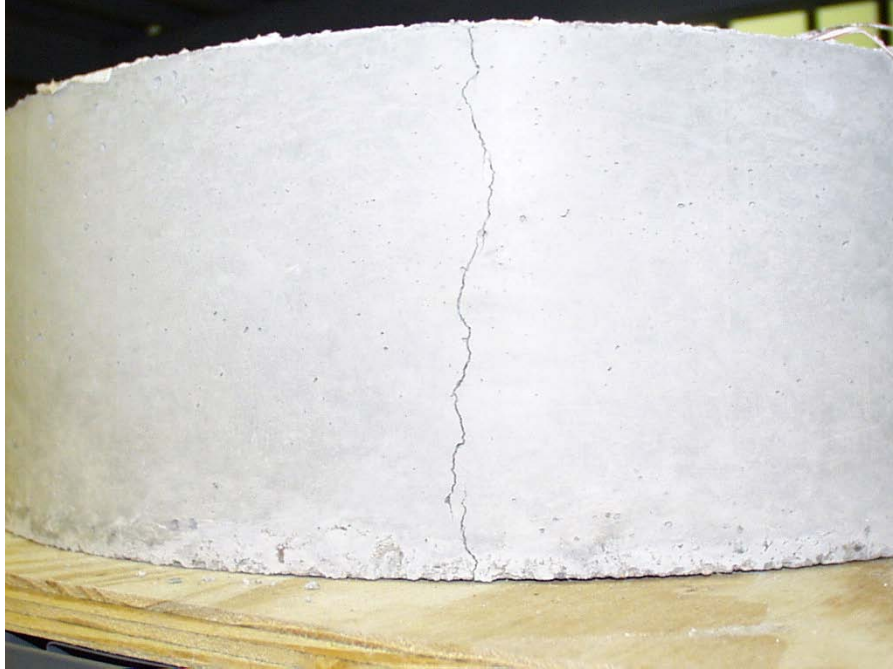
Figure 3.38 Large Crack in Restrained Shrinkage Ring Specimen
