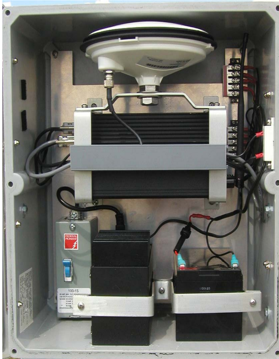
Figure 4.6: GPS Hardware Package (cover removed)
