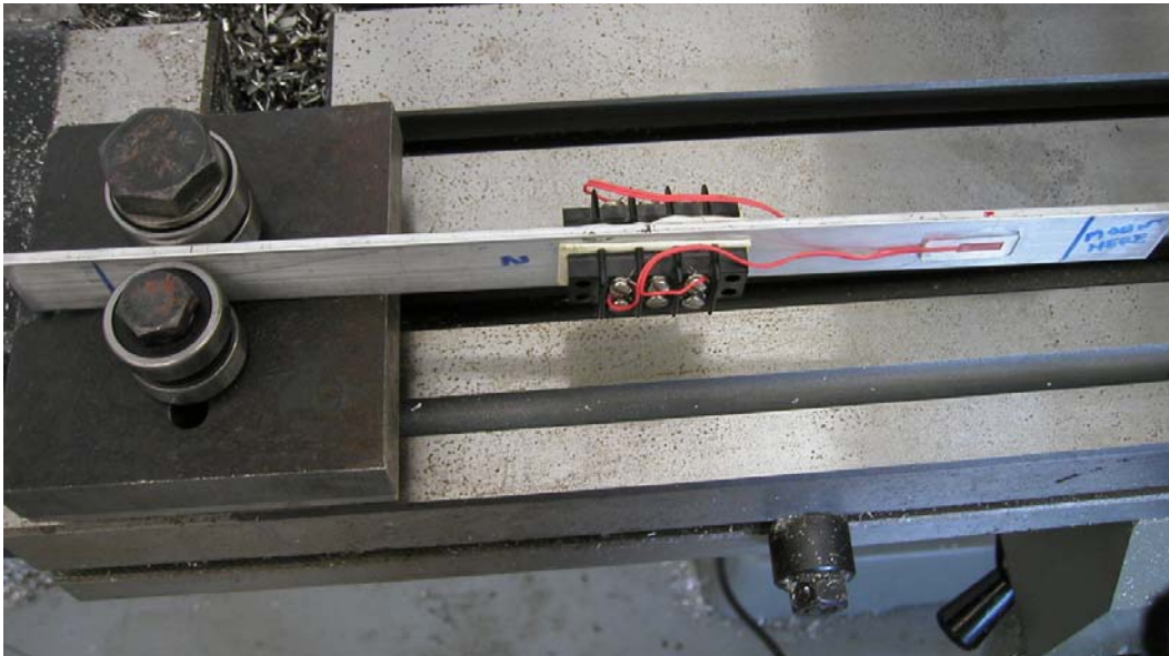
Figure 2.14: Test Beam on CNC Milling Machine
