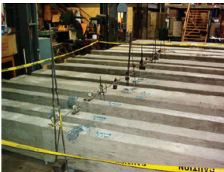
Figure 3: Monitoring of Camber
