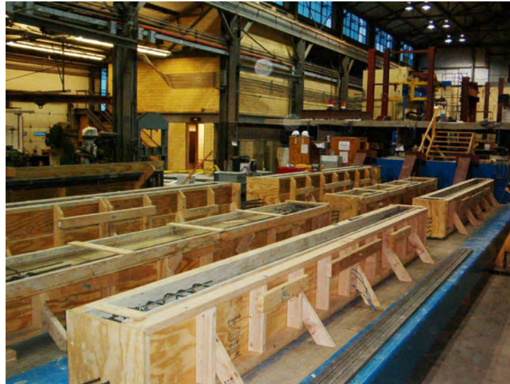
Figure B.2: Prestressing bed at Ferguson Laboratory 2
