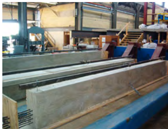
Figure 4-8: Optimized configuration with one potentiometer per beam
