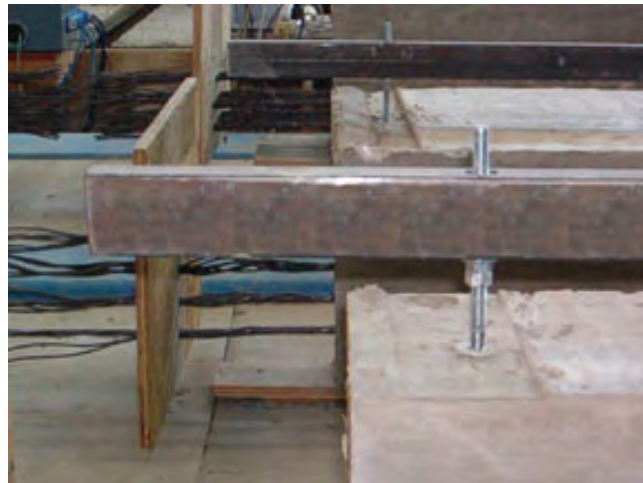
Figure 4-10: Support of frame for camber measurement
