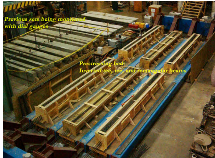
Figure B.1: Prestressing bed at Ferguson Laboratory
