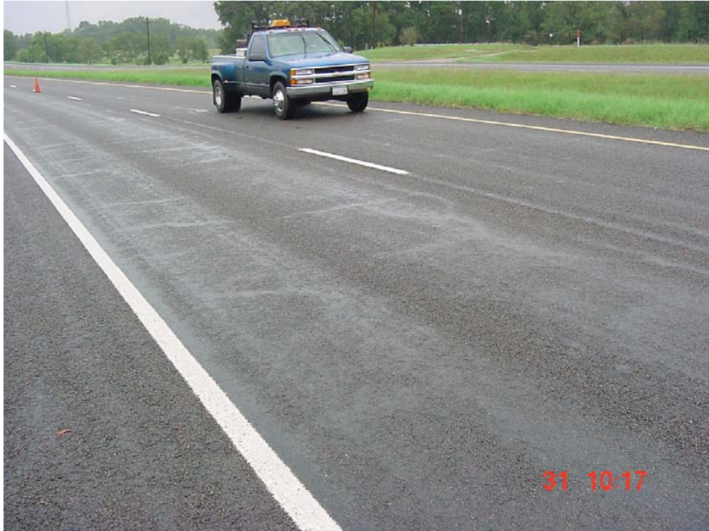
Figure 4.4. Test section crack sealed with H1 in Atlanta District
