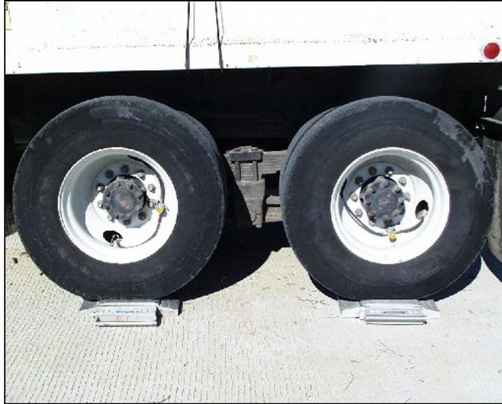
**Figure 5.4 Weighing of Back Axles**
