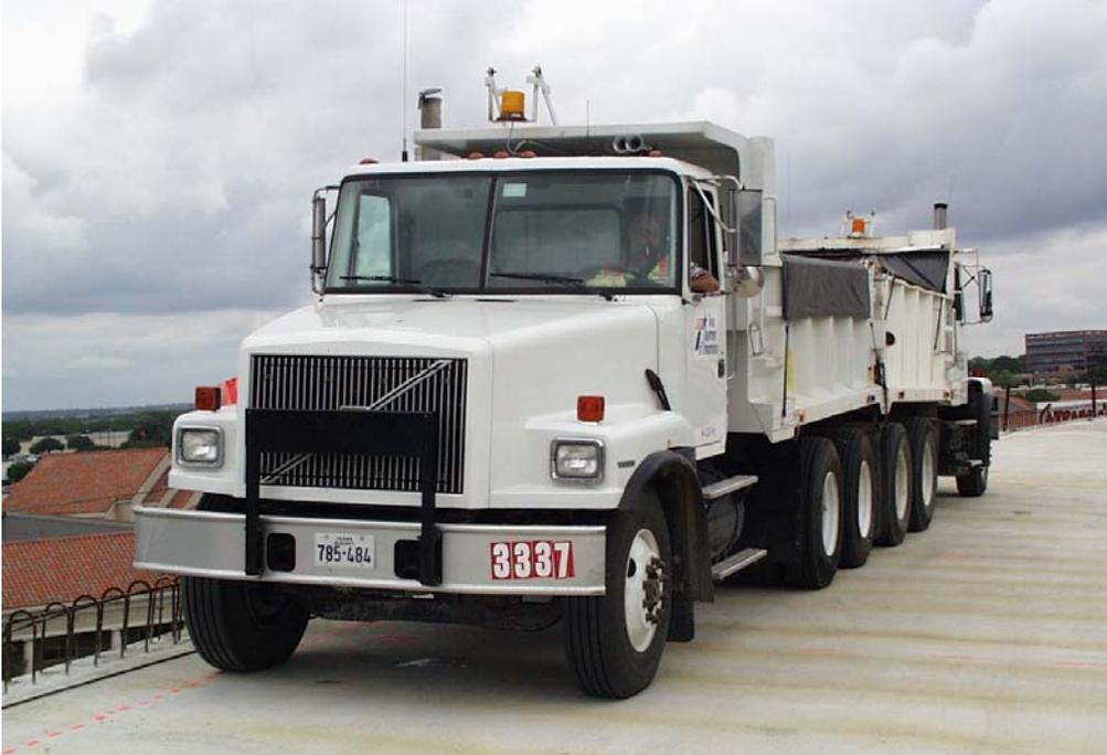
**Figure 5.7 Truck Positioning during K Live Load Test**
