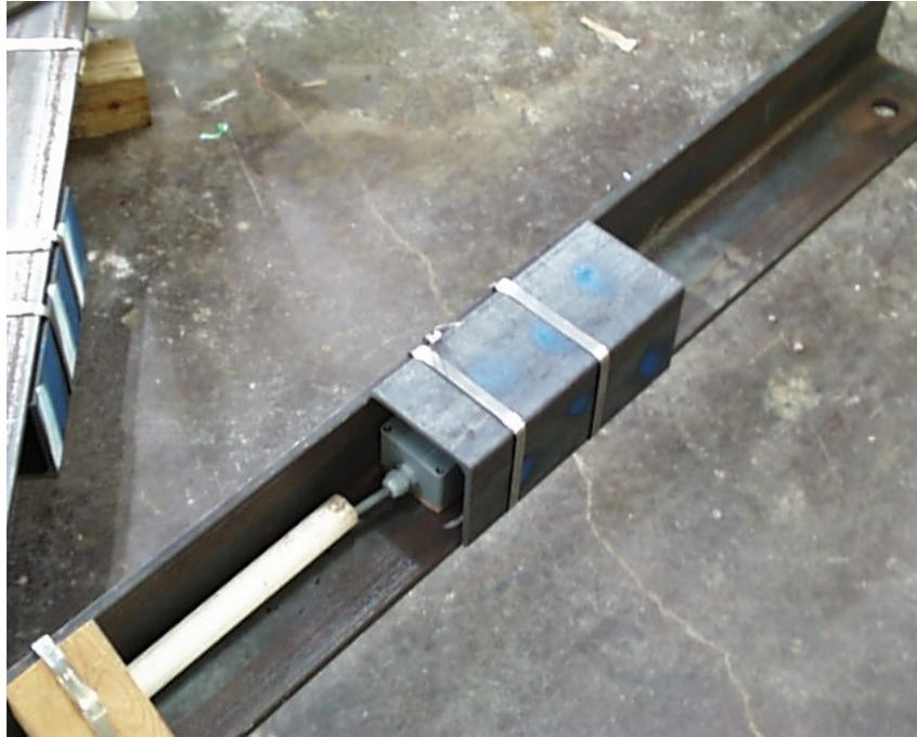
**Figure 2.4 Instrumentation Protection**
