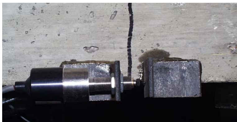
Figure 5.17 Displacement Transducer used to Opening and Closing of Flexural Crack
