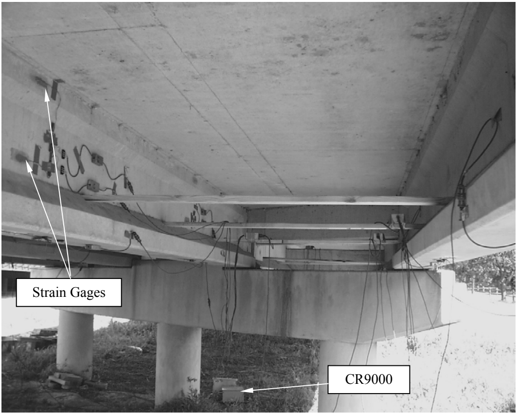
Figure 3.13 Instrumentation Used to Monitor Bridge Response during Diagnostic Load Tests
