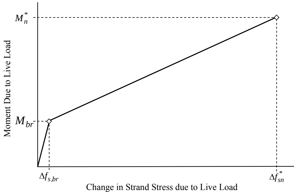
Figure 9.10 Idealized Bilinear Relationship between Live Load Moment and Strand Stress Range
