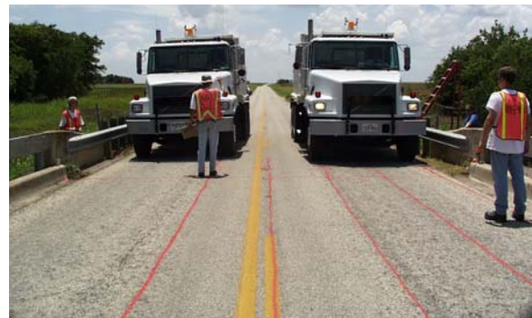
Figure 3.6 Side-by-Side Trucks on Willis Creek Bridge
