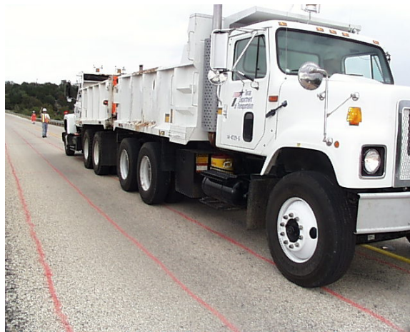
Figure 3.8 Back-to-Back Trucks on Lampasas River Bridge
