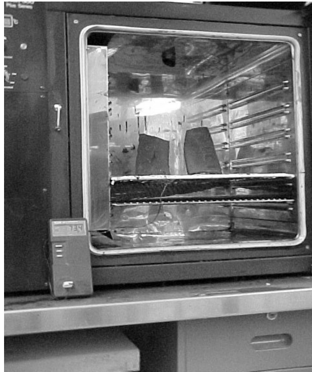
Figure E-5 Tire Sidewall Pieces with Imbedded Thermo-couple Sensor in Oven
