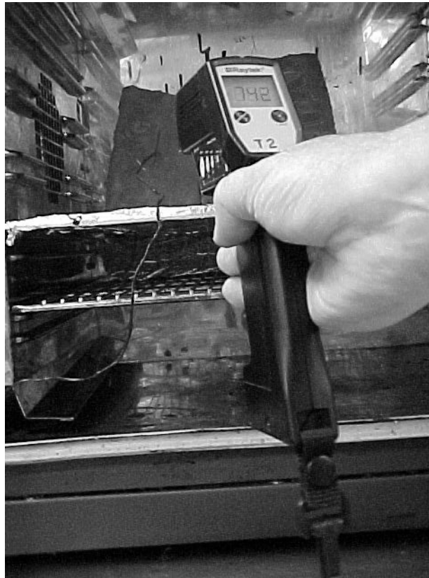
Figure E-6 Measuring the Temperature of the Tire Sidewall Piece inside Oven with Infrared Thermometer
