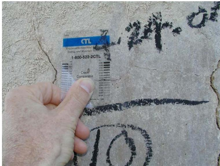
Figure 6.10: Crack comparator card
