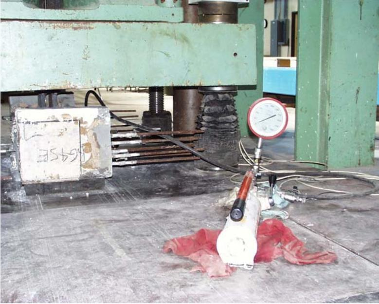
**Figure 3.29: Slice specimen in loading machine for strand-pullout tests**
