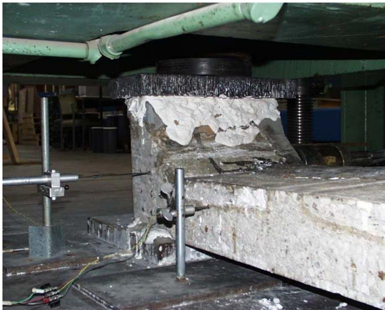
Figure 3.31: Steel plate between loading head and slice specimen
