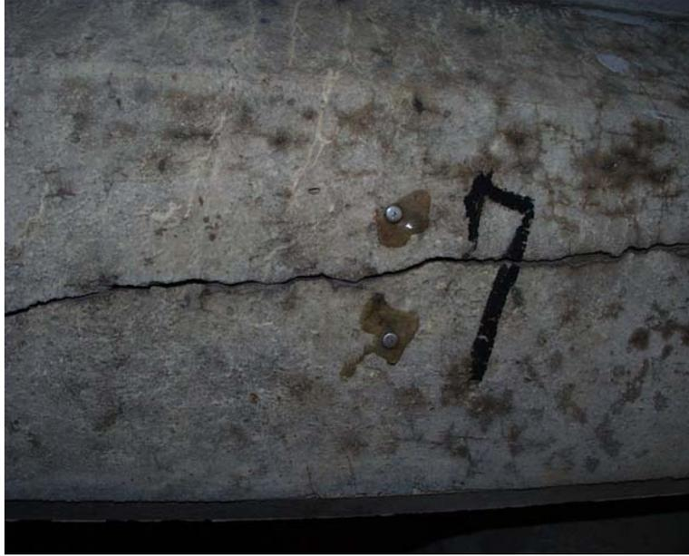
**Figure 6.13: One set of Demec discs for monitoring crack width**
