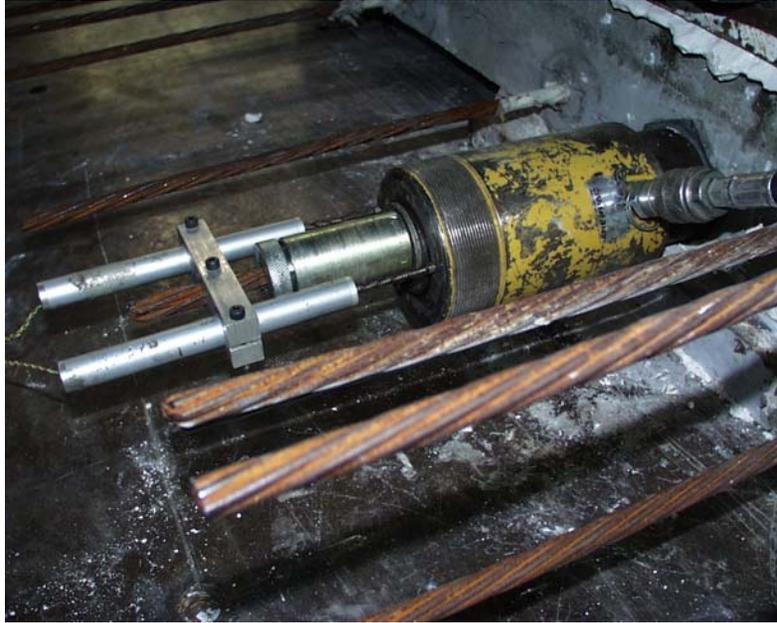
**Figure 3.33: Linear potentiometers at loaded end**
