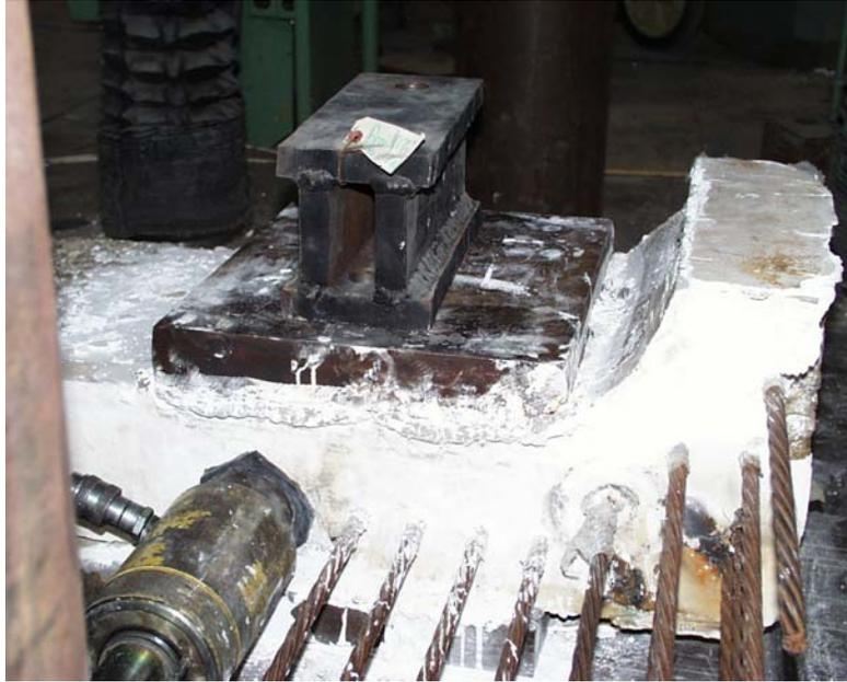
**Figure 3.32: Steel spacer and plate used for middle strands**
