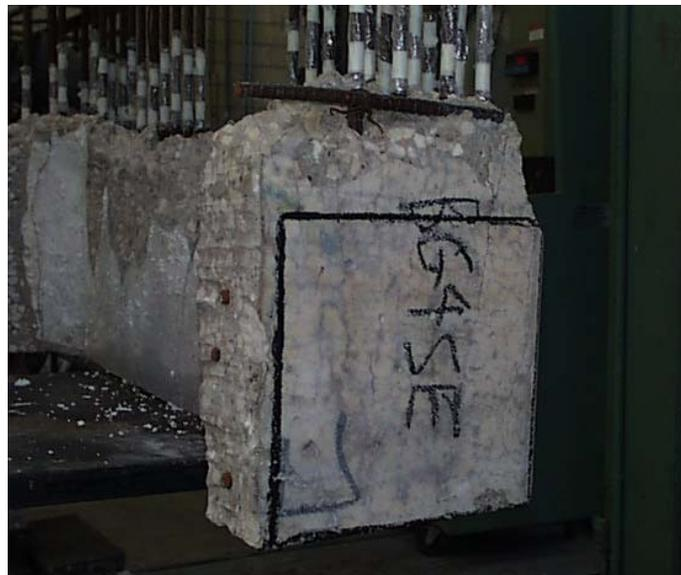
**Figure 3.37: Representative square for left side damage index**
