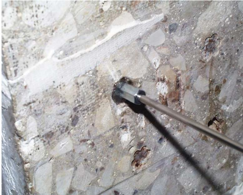
**Figure 3.34: Linear potentiometer attached to back of strand**
