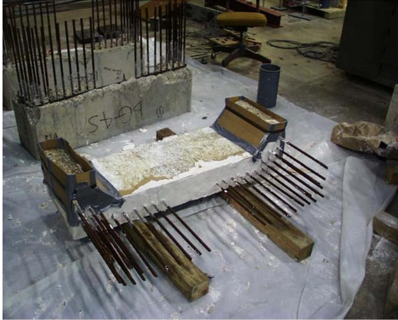
**Figure 3.25: Formwork for web sections**
