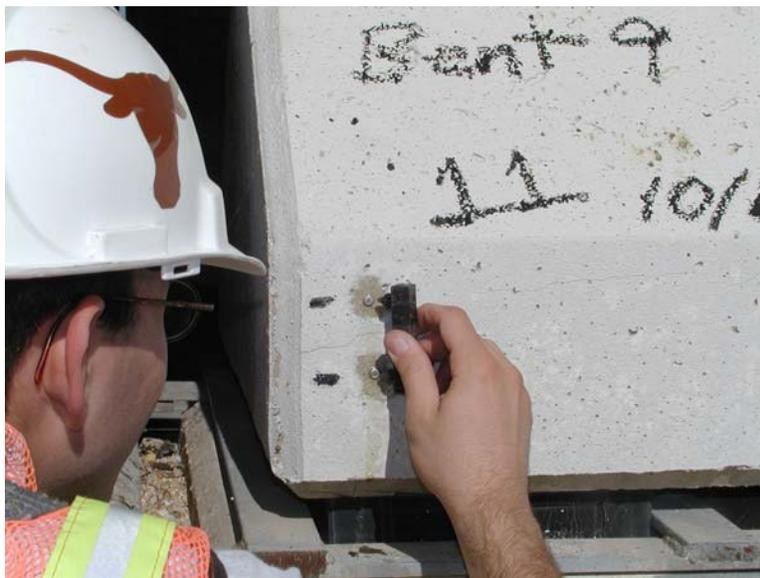
**Figure 6.14: Holding set of Demec discs in place with reference bar**
