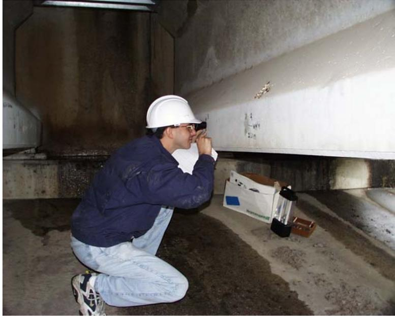
**Figure 6.11: Measuring crack widths with optical scope**
