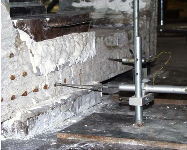
**Figure 3.35: Linear potentiometers recording relative movement of strand at free end**
