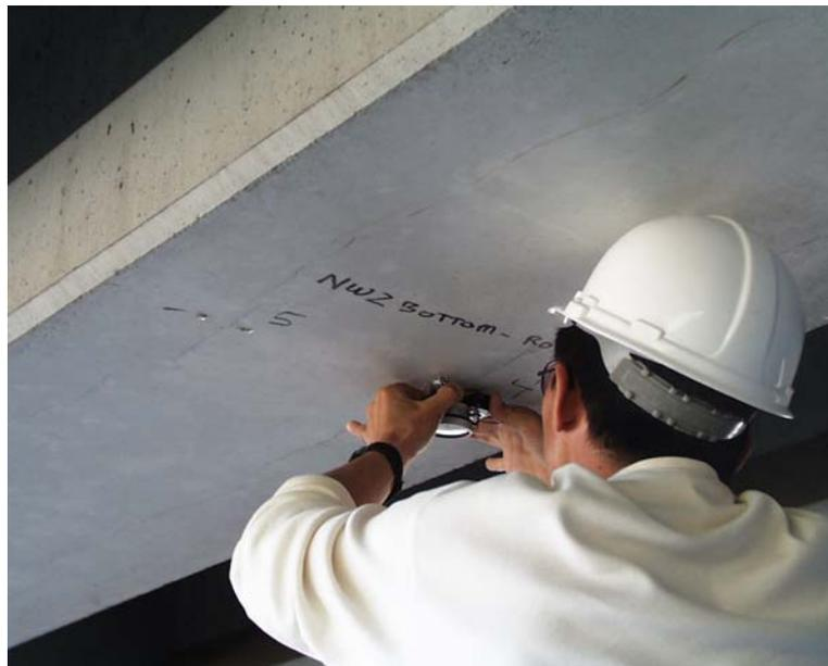
**Figure 6.12: Taking readings with Demec gauge**
