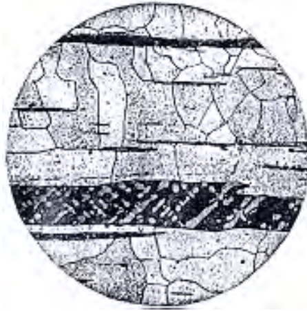
Figure C.1: Longitudinal section of wrought iron
