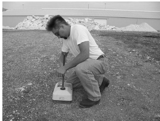
(b) Nuclear density testing on subgrade
