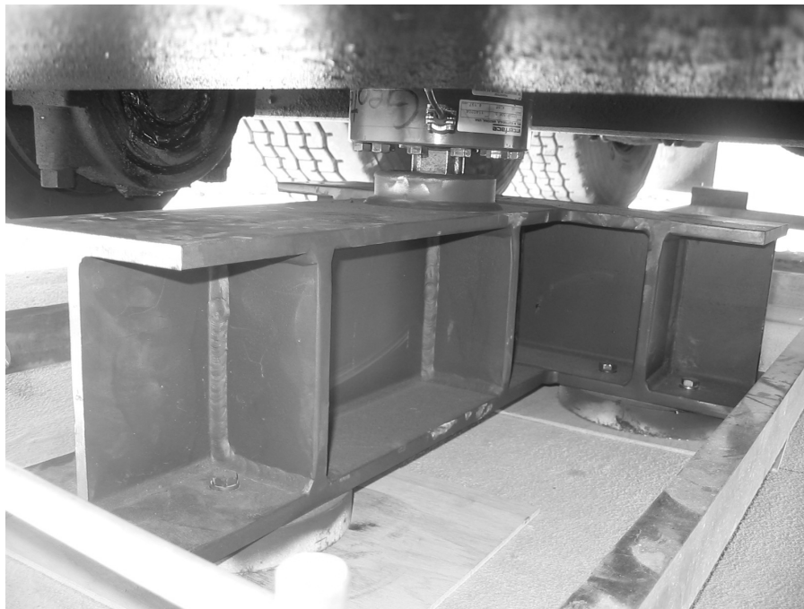
(b) Loading mechanism in position over loading frame
