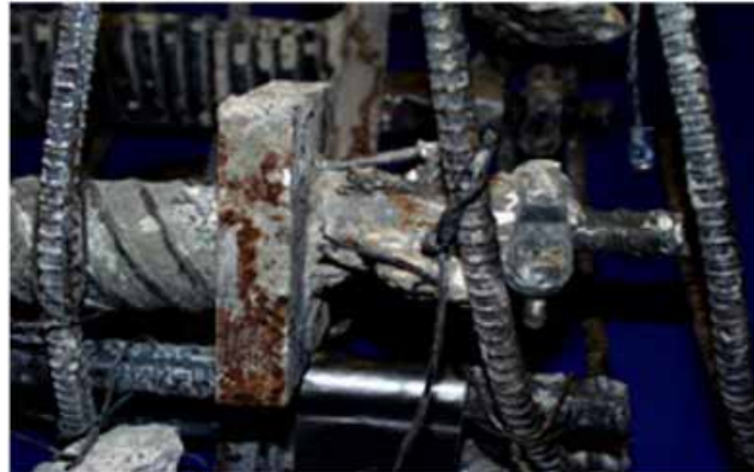
Figure 4.19 PT Bar Top Anchorage Condition for Specimen PT-TC-N-PD¹
