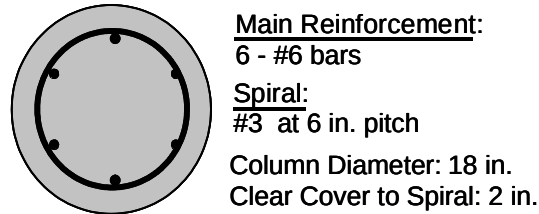
Figure 2.2 Reinforced Concrete Column Section Details 2
