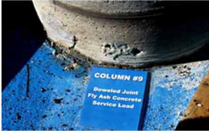
Figure 4.11 Condition of Specimen DJ-FA-S at the End of Testing 1
