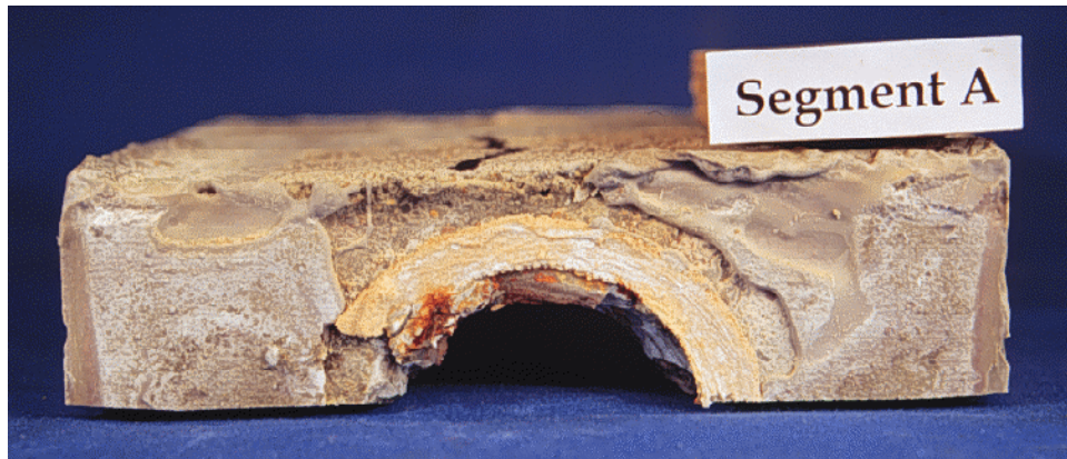
Figure 4.18 – Incomplete Epoxy Coverage in Epoxy/Gasket Joint (EG-S-M-NG-2)
