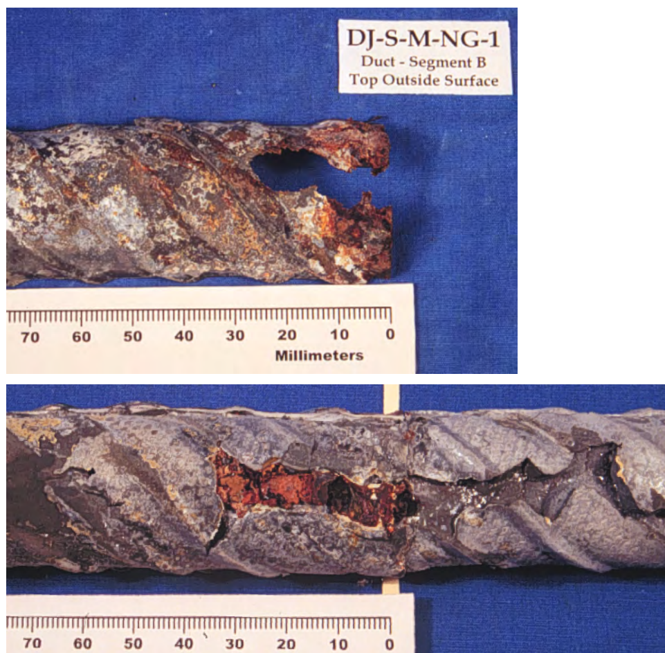
Figure 5.6 – Hole in Duct Corresponding to Grout Void
