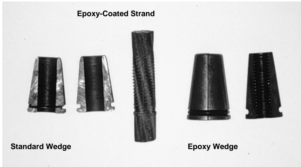
Figure 2.37 - Comparison of Post-Tensioning Wedges
