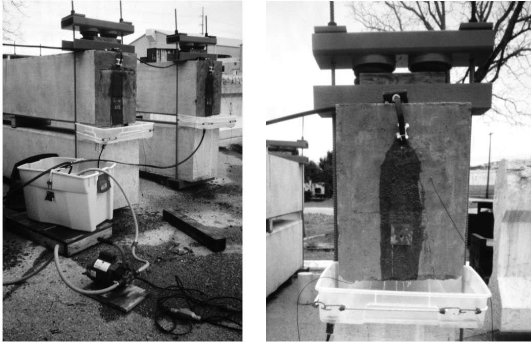
Figure 2.28 - Beam End Drifter System
