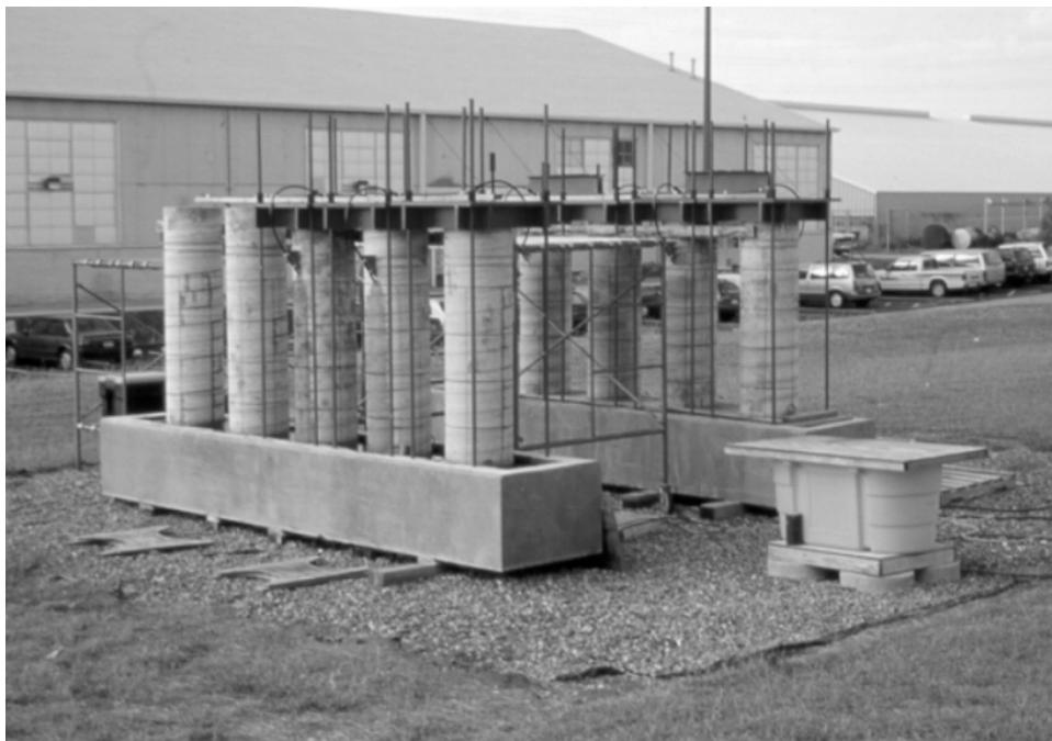
Figure 3.10 - Long-Term Column Corrosion Test Setup
