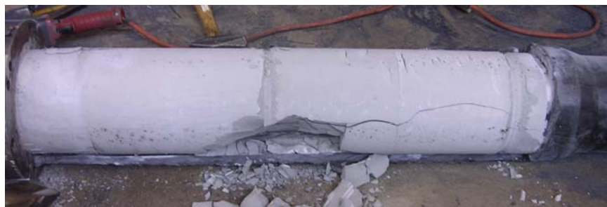
Figure D.135 Condition of Grout near Deck End – Specimen 11
