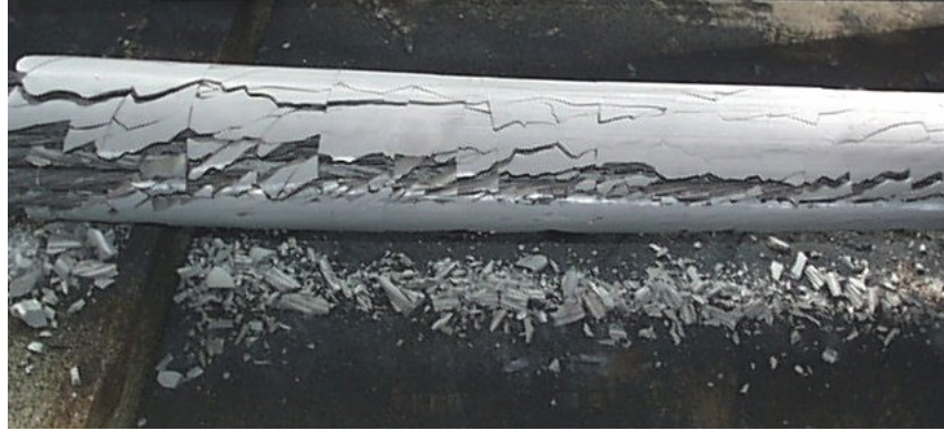
Figure D.121 Condition of Grout at Midspan Immediately after Removing PE Pipe – Specimen 10
