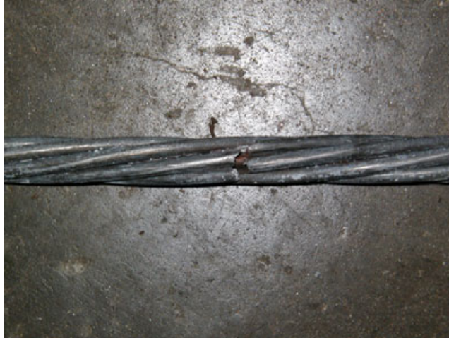
Figure E.8 Wire Breaks near Midspan – Specimen 1
