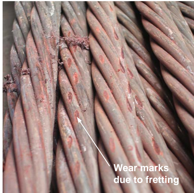
Figure 3.19 Reduction of Cross-Sectional Area of Strands Due to Fretting – Specimen 8
