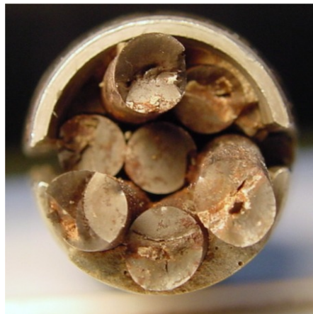
Figure D.26 Fracture Surfaces for Strand 2 near Tower End – Specimen 2
