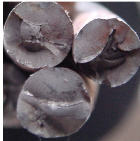
Figure D.16 Fracture Surfaces for Strand 19 at the Tower End of Specimen 1
