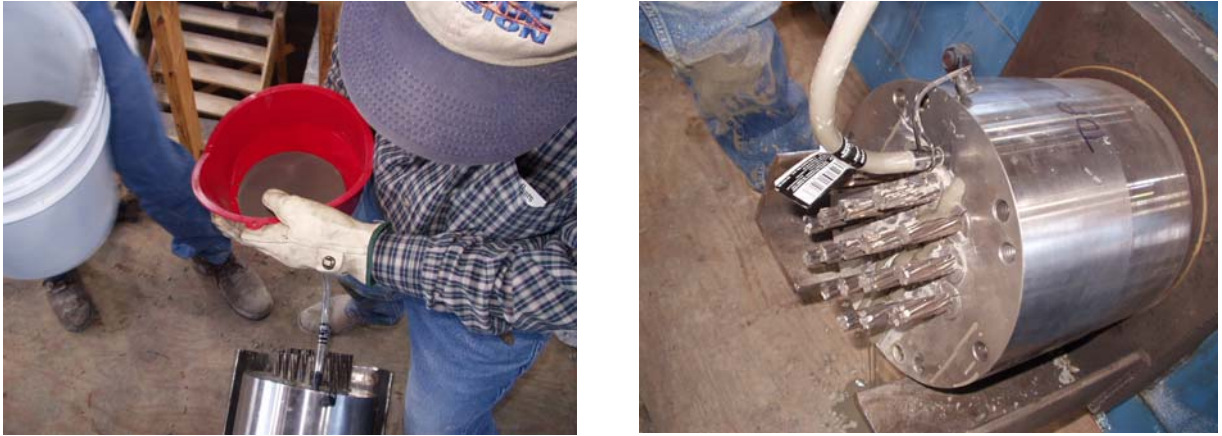
Figure B.39 Procedure Used to Fill the Intentional Grout Void at the Tower End of Specimen 9
