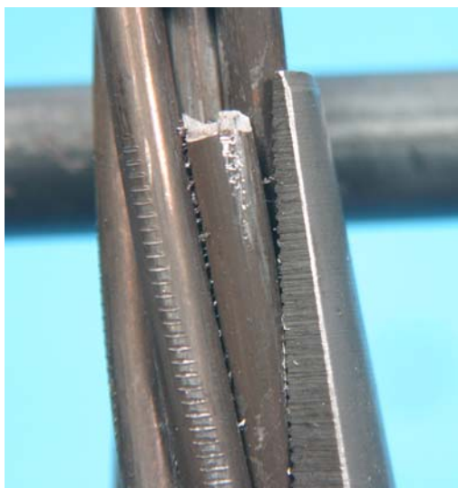
Figure D.96 Wire Breaks in Strand 9 at Wedge near Tower End – Specimen 8
