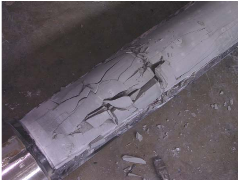
Figure D.120 Condition of Grout at Tower End Immediately after Removing PE Pipe – Specimen 10
