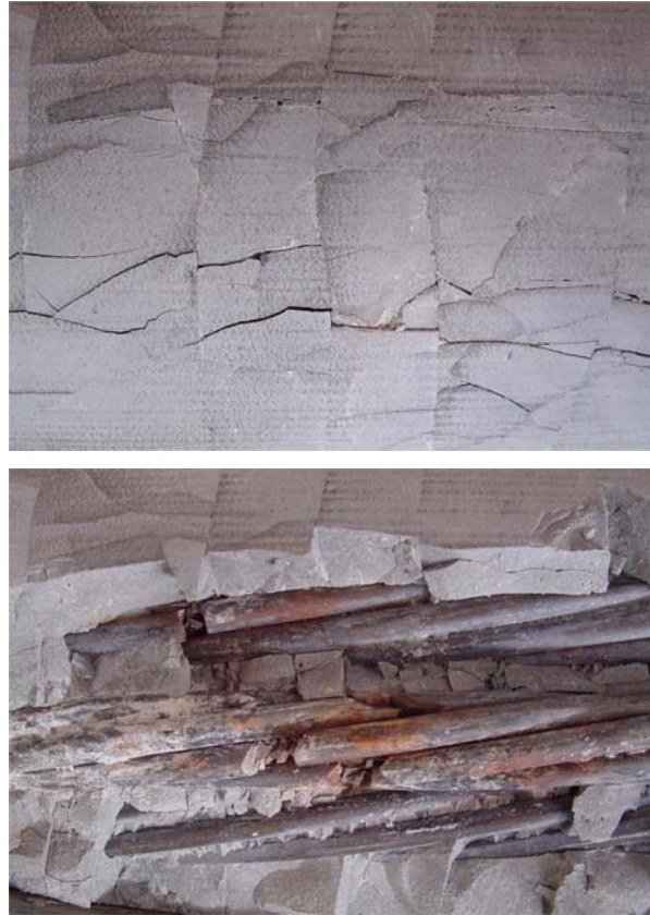
Figure D.8 Longitudinal Cracks in Grout, Corrosion of Strand, and Wire Breaks near Midspan of Specimen 1
