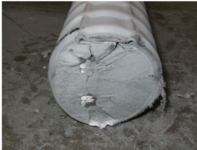
Figure E.9 Typical Vertical Crack in Grout – Specimen 1
