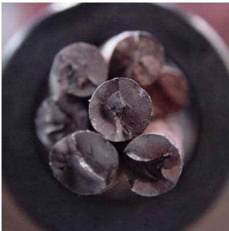
Figure D.16 Fracture Surfaces for Strand 19 at the Tower End of Specimen 1
