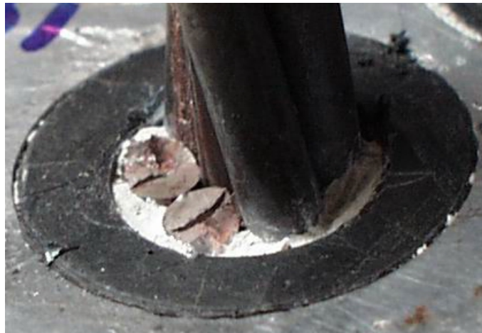
Figure D.66 Wire Breaks in Strand 17 at the Inside Face of the Tower Anchor Hear – Specimen 6
