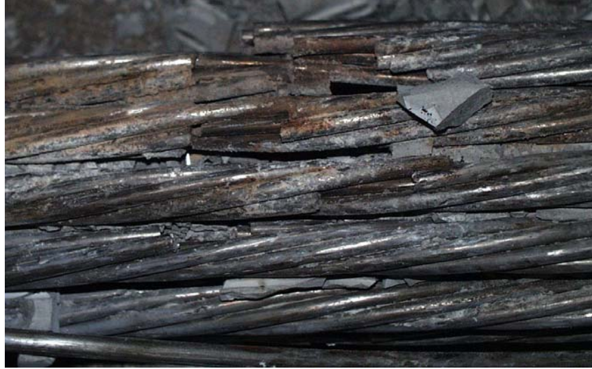
Figure 3.9 Corroded Fretting Product on Surface of Strand at Midspan – Specimen 12
