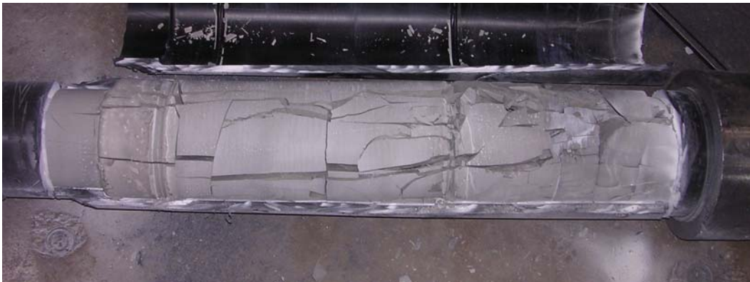
Figure 3.10 Condition of Grout at Deck End Immediately after Removing PE Pipe – Specimen 10
