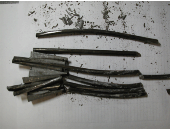
(c) Wire Breaks in Bottom Strand inside Anchor Head
