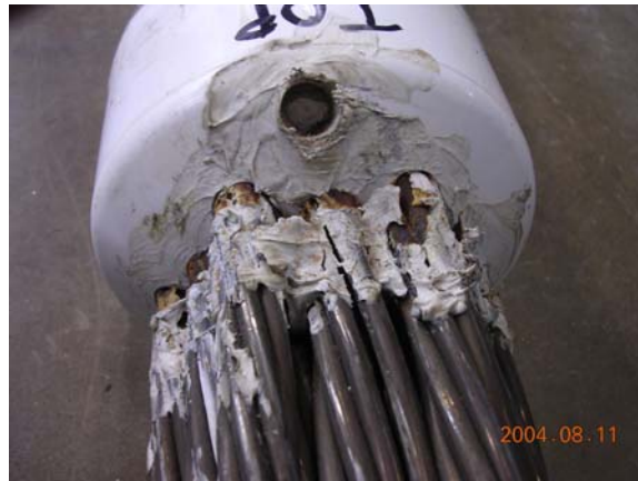
Figure D.137 Corrosion at Interface between Grout and Caulk near Midspan – Specimen 11
