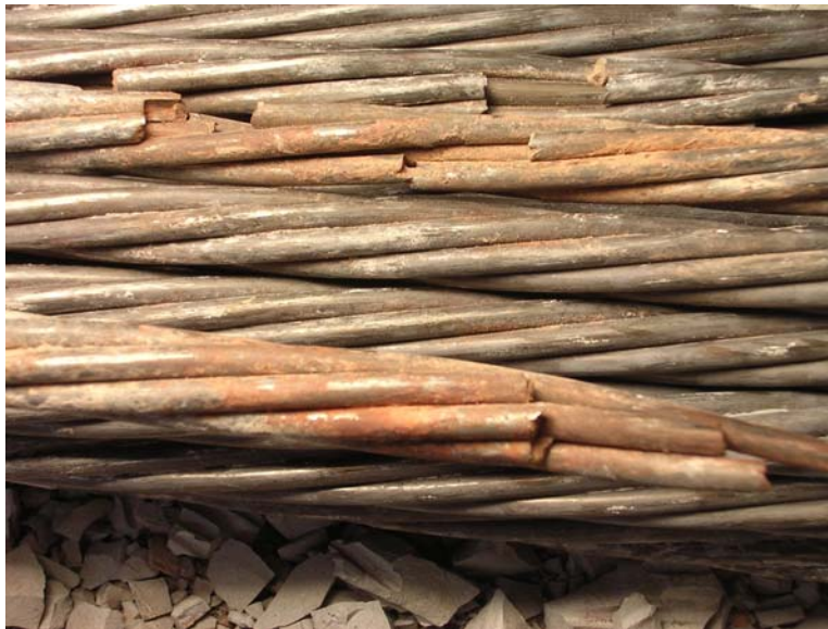
Figure D.109 Corrosion on Surface of Strand near Midspan – Specimen 9
