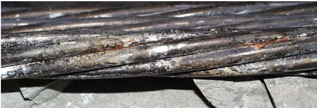
Figure D.61 Corrosion on Strand 19 near Tower Anchor Head – Specimen 6
