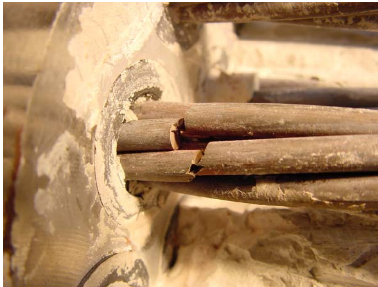
Figure D.14 Wire Breaks in Strand 2 near Tower End of Specimen 1
