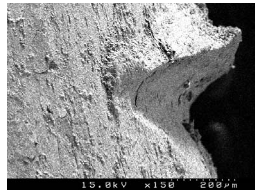
Figure D.33 Typical Tooth Mark
