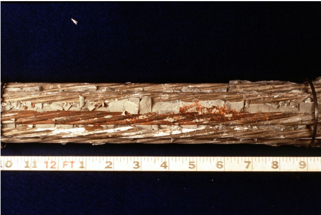
Slide 9. Corrosion product on surface of grout during accelerated corrosion test (Specimen LS-5 opening 5).
