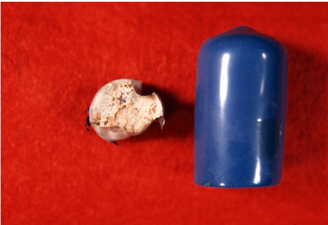
Slide 125. Grout in epoxy repair cap. February 20, 1995.
