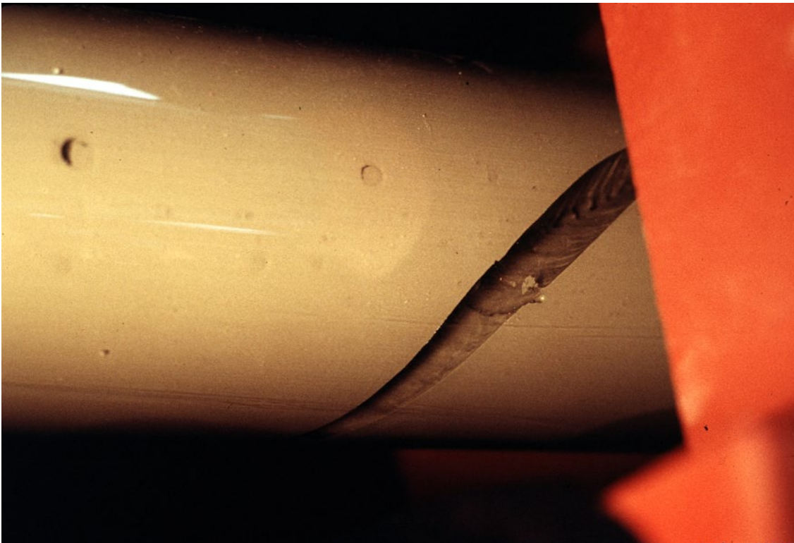
Slide 97. Large scale test one (LS-1). Break in grout at bott [?] trans. in third after grout.
