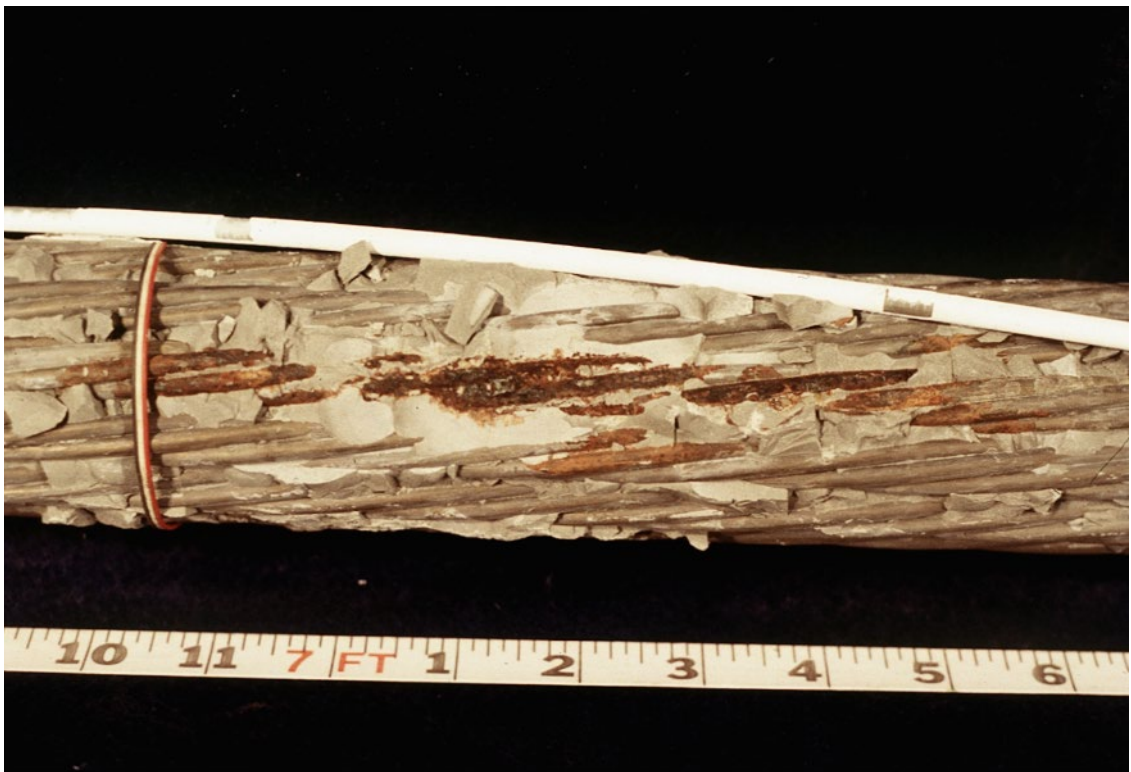
Slide 116. Large scale test one (LS-1). Corrosion. 2nd copy. March 28, 1994.
