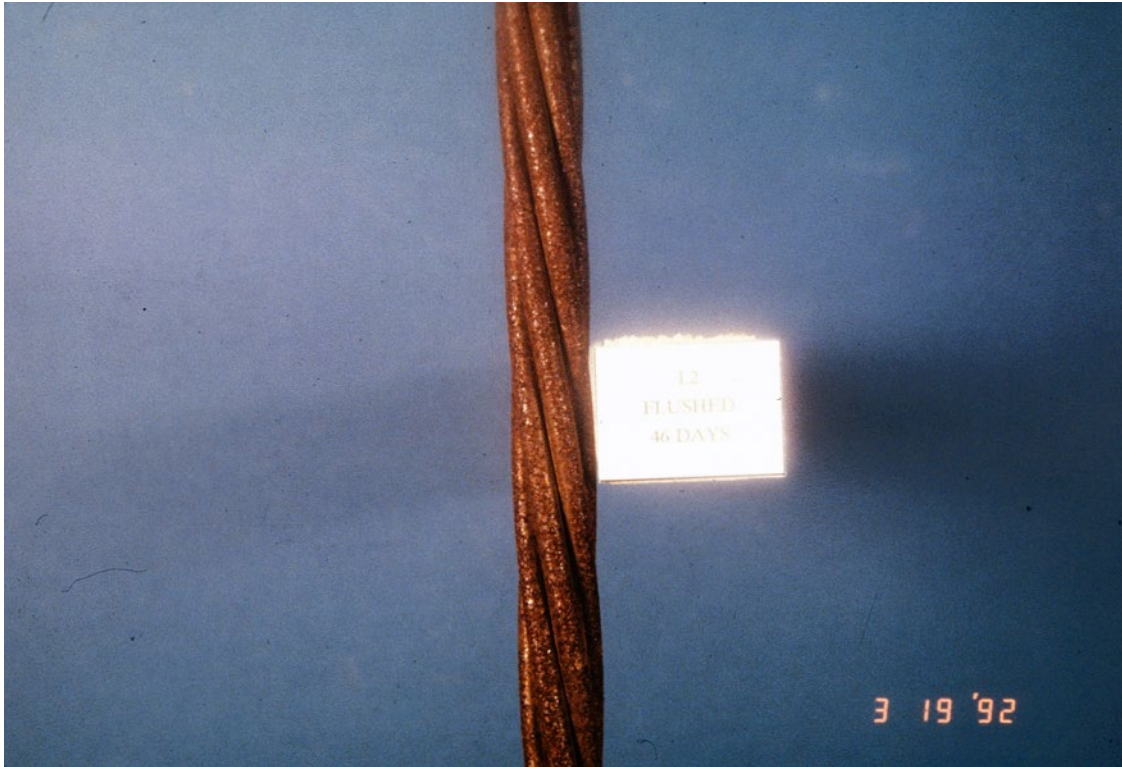
Slide 176. Lubricant two (L2). Flushed 46 days. March 1992.
