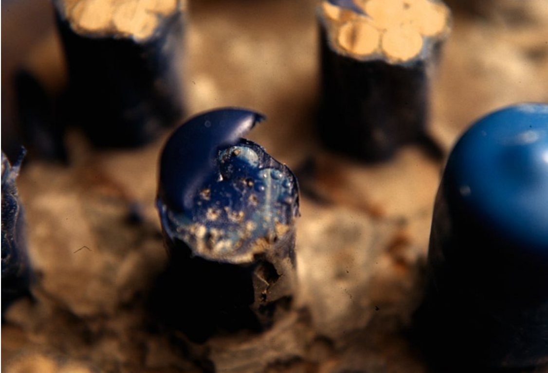
Slide 60. Large scale test six (LS-6). Moisture visible. December 14, 1994.
