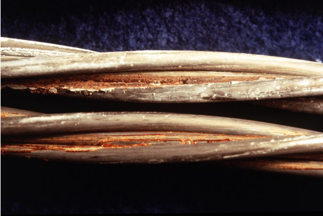
Slide 10. Corroded metal strand.
