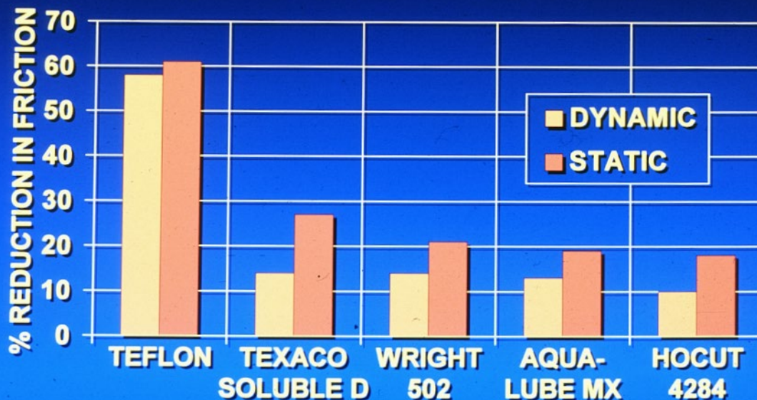
Slide 159. Reduction of Dynamic and Static Friction in Small-Scale Test
