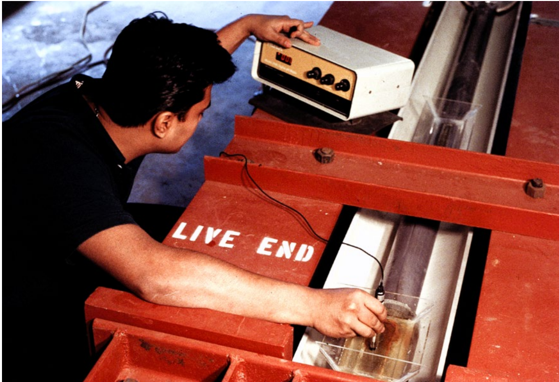
Slide 50. Large scale specimen – half-cell potential measurement. February 2, 1994.
