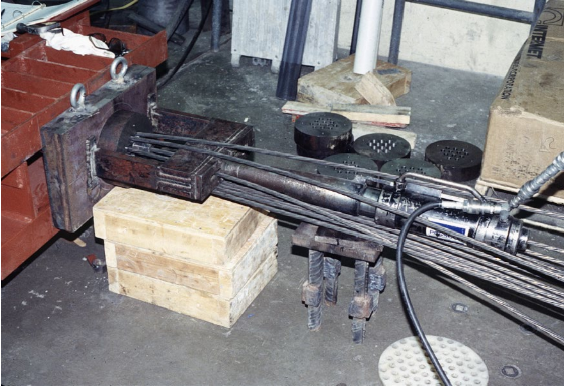
Slide 83. Large scale test three (LS-3). Assembly. Dead end stressing assembly.
