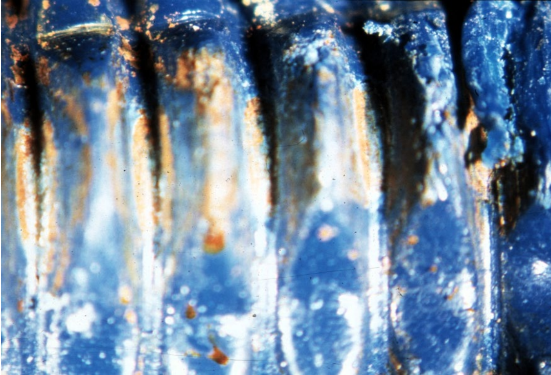
Slide 64. Corrosion of strand at tooth mark.
