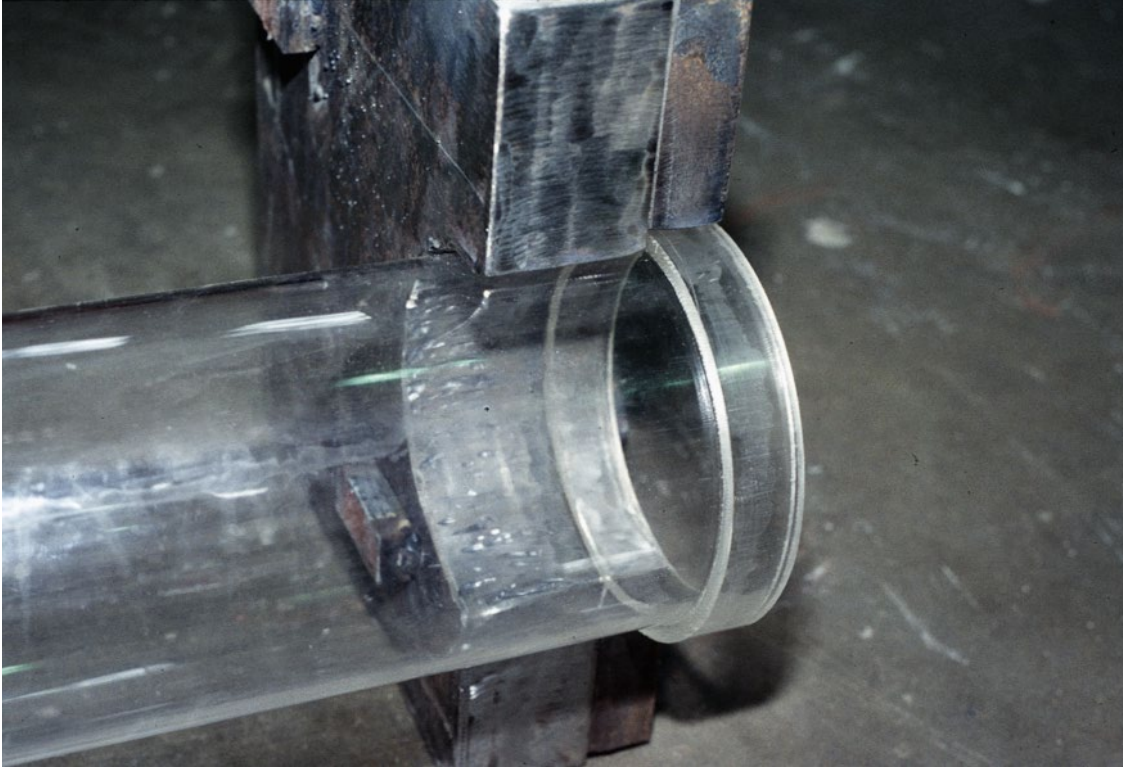
Slide 81. Large scale test three (LS-3). Assembly. Dead end transition pipe and plate.
