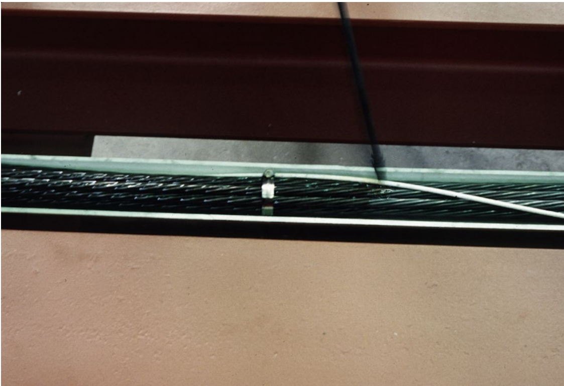
Slide 82. Large scale test three (LS-3). Installation. Coating strand with oil.
