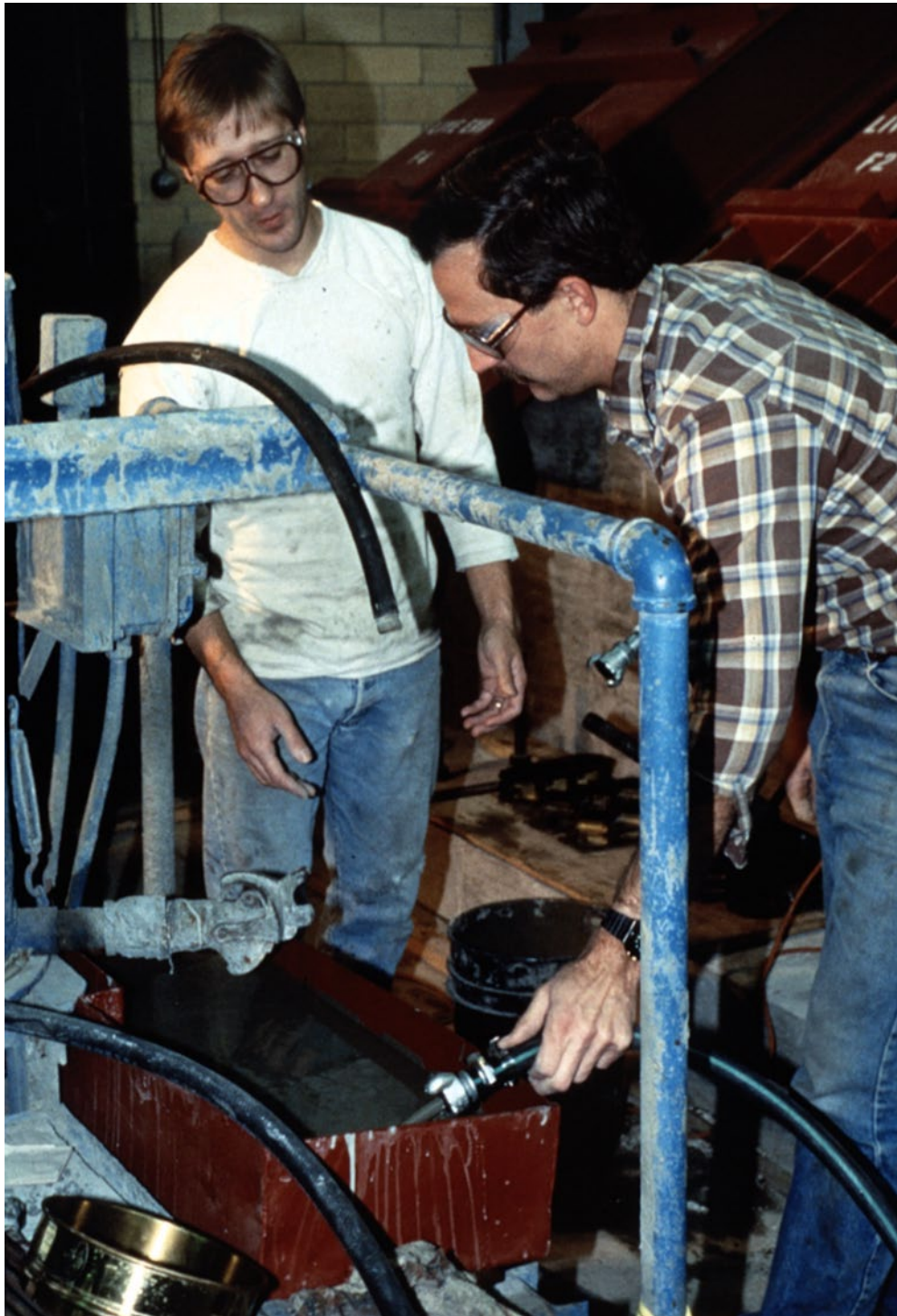
Slide 89. Recirculating to remove air.
