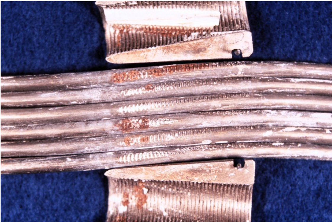
Slide 11. Corrosion at the interface between the strand and wedge and between tooth marks.
