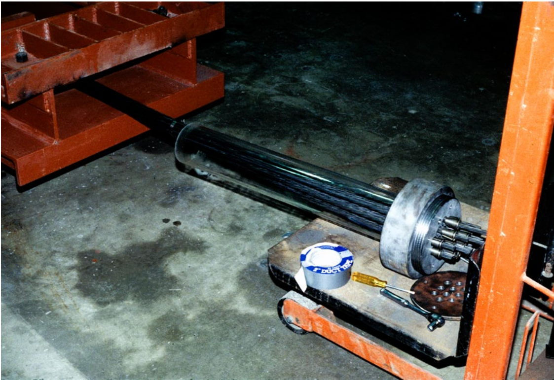
Slide 78. Large scale test three (LS-3). Assembly. Installation of live end anchor head.
