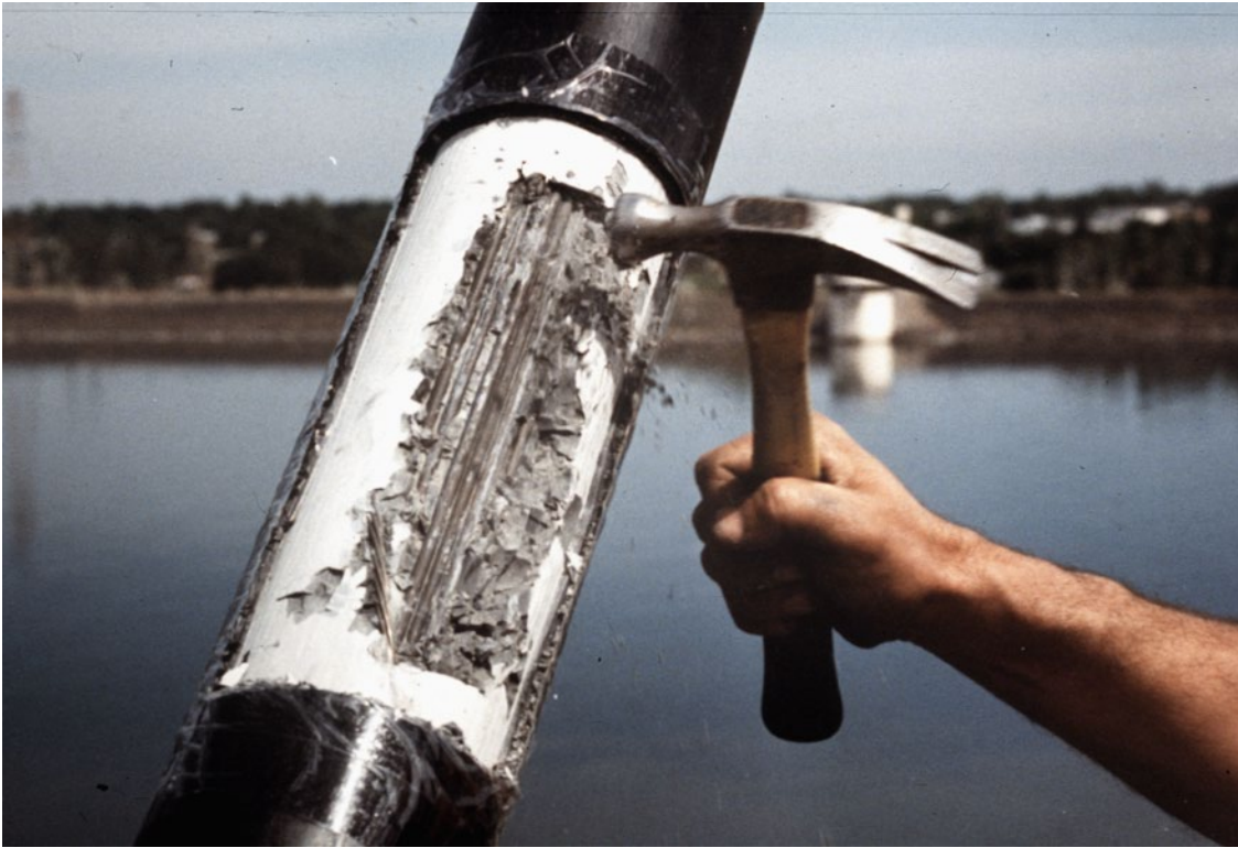
Slide 75. Breaking open stay cable.
