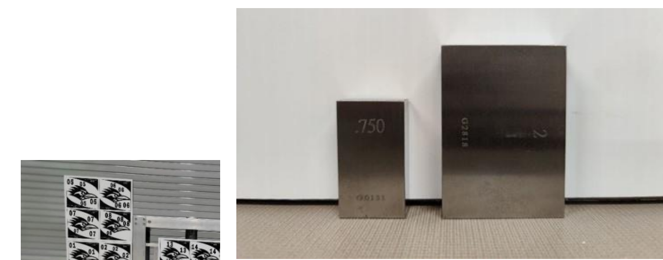
Gage block device NIST certified gage blocks
